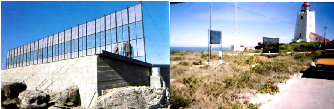
**Figure 2-6: Left: Fog Water Collection System (FWCS) at Mariepskop (1969) (Schutte, 1971). Right: Test fog water collectors at Cape Columbine lighthouse during the research that was conducted in 1995. The ‘standard’ 1 m<sup>2</sup> fog water collector is shown to the left. The larger test system on the right was donated by a private individual (Maarten van Schoor) and was only deployed at Cape Columbine [10].**
