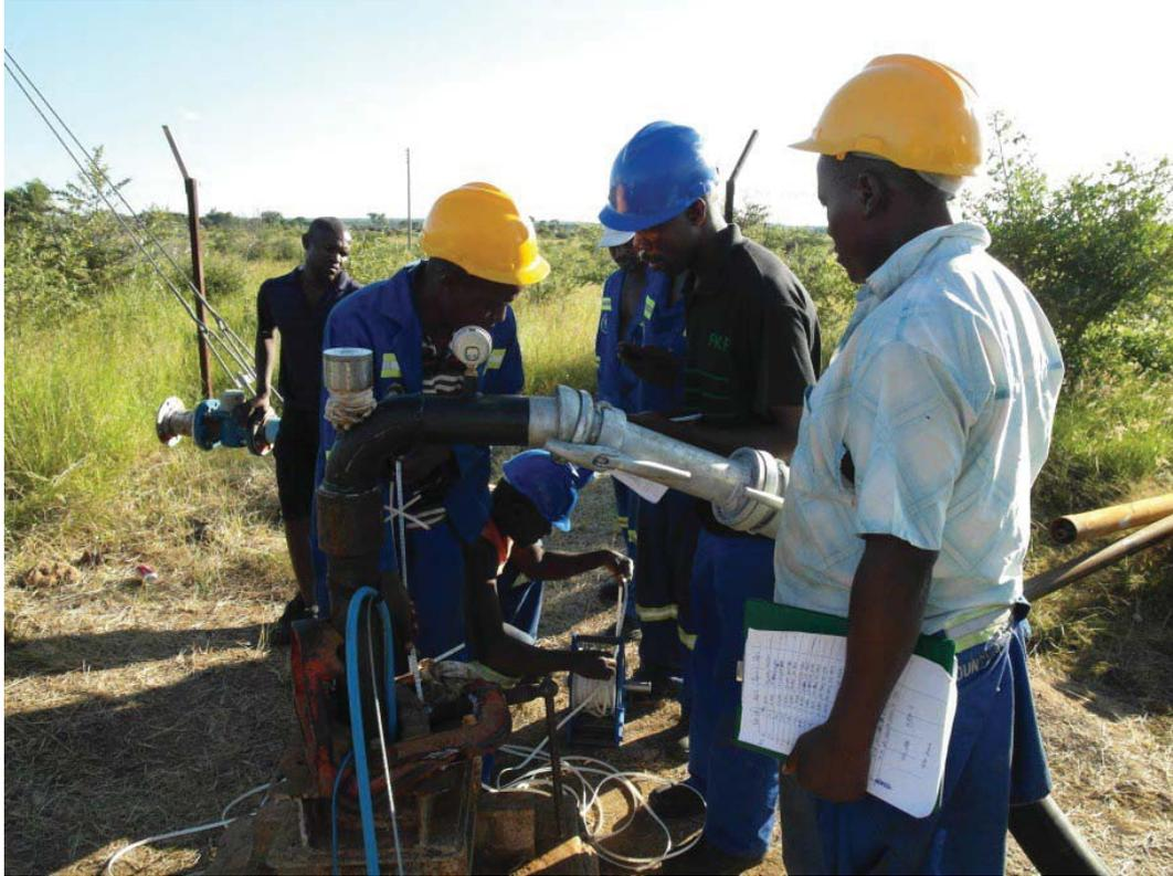
**Figure 15: Taking water level readings**
