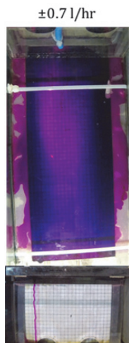
Figure 6-10. Screenshots of the horizontal fracture and vertical wall for the continuous flow experiment at each interval during the test, under 1G conditions (5 mm x 5 mm grid).
