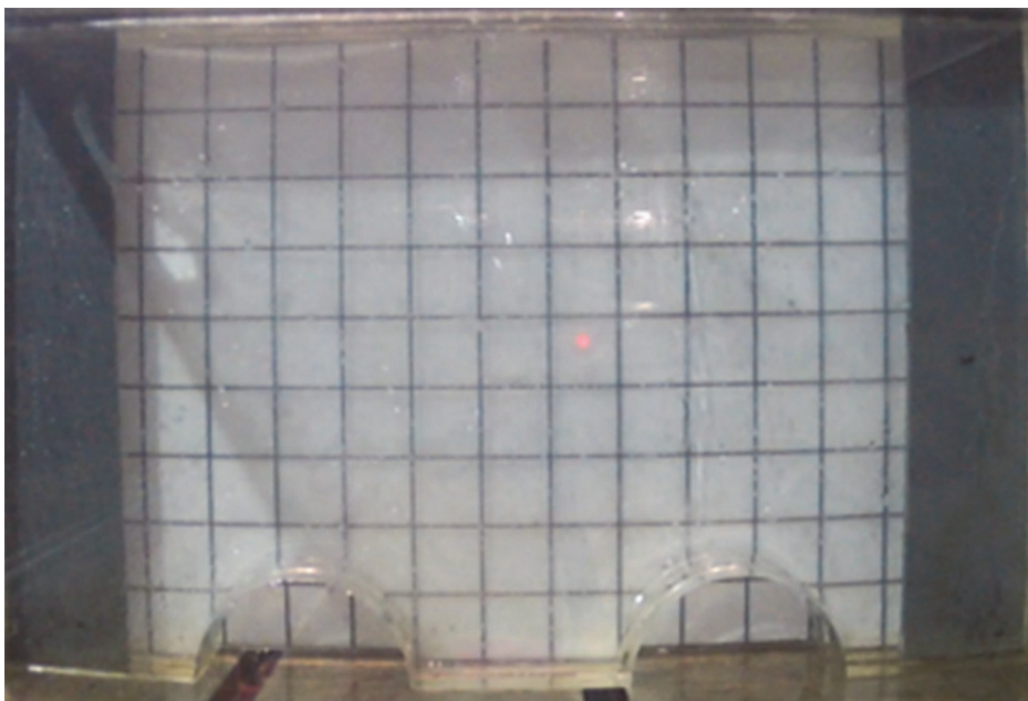
Figure B-9. Drying of the vertically inclined fracture during the 20G test.
