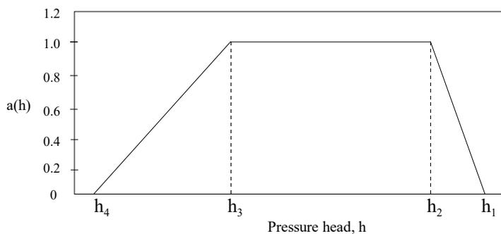
Figure 4.5 Schematic of the plant water stress response function  $a(h)$  and soil matric pressure head,  $h$ , as used by Feddes *et al.*, 1974.
