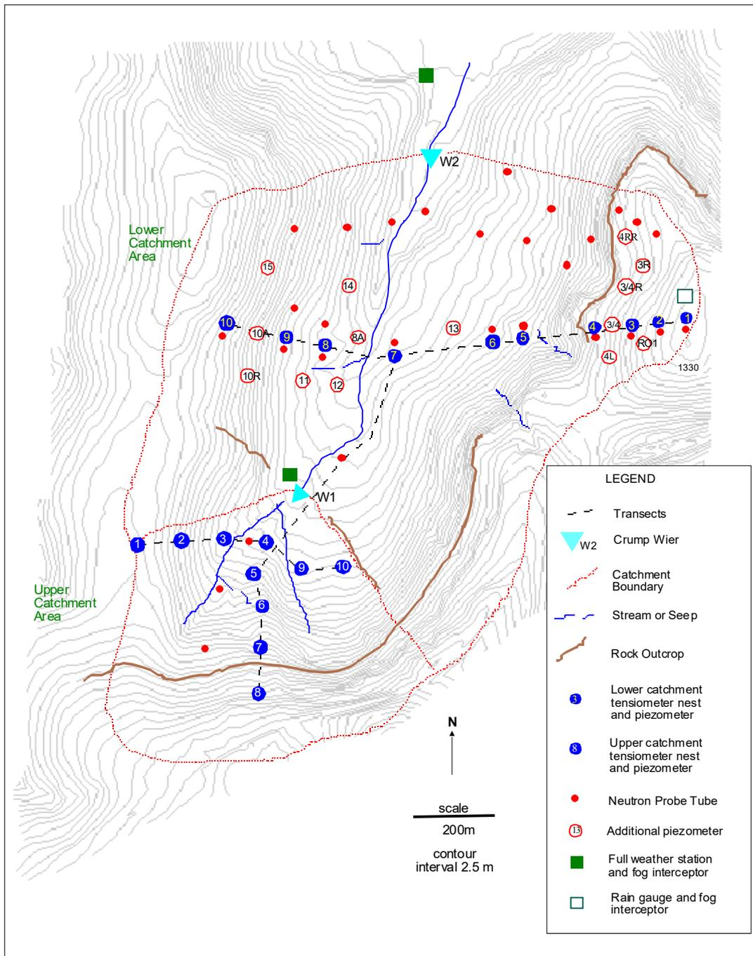
Figure 3.1 Layout of the Weatherley research catchment, showing the location of monitoring and instrumentation stations.
