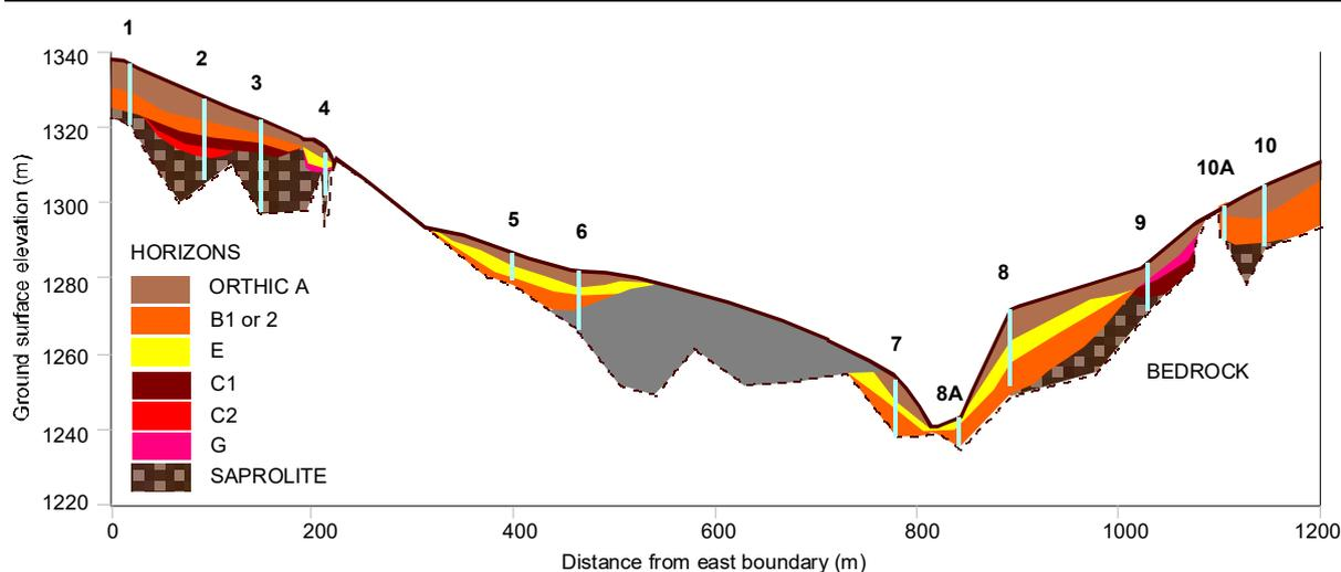
Figure 3.2 Cross section of transect 1, showing soil and bedrock profile.
