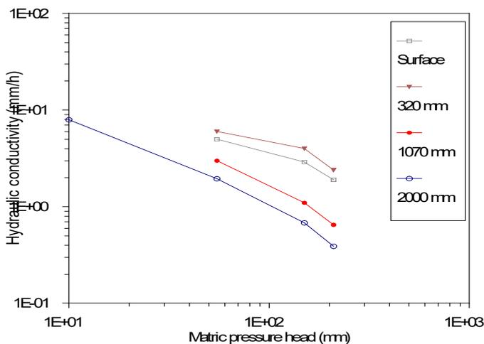
Figure 4.7 Hydraulic conductivities for the Taylors Halt profile. (The double ring infiltrometer, saturated hydraulic conductivity is plotted at a matric pressure head: 10 mm)
