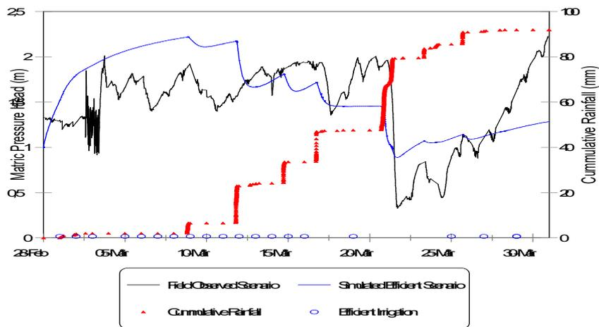
Figure 4.12c. Simulated proposed efficient scenario and observed matric pressure heads at Taylors Halt, nest 1 at a depth of 0.2 m.
