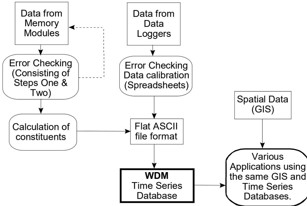
Figure 2.3. Data Flow diagram for integration of time series in WDM format and GIS.
