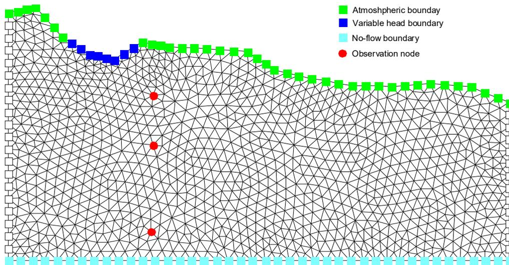
Figure 4.4 HYDRUS-2D finite element grid of the soil profile at nest 2 of the Willowfontein site.
