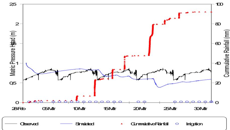
Figure 4.12b. Simulated and observed matric pressure heads for current practice at Taylors Halt, nest 1 at a depth of 0.72 m.
