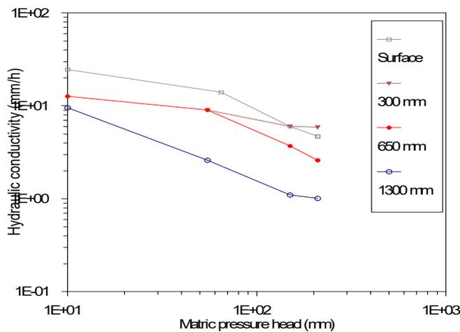
Figure 4.6 Hydraulic conductivities for the Willowfontein profile. (The double ring infiltrometer, saturated hydraulic conductivity is plotted at a matric pressure head: 10 mm)
