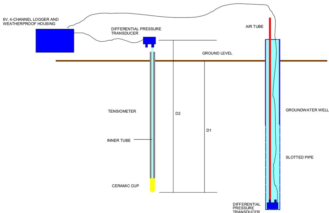
Figure 3.4 Automatic tensiometer and groundwater level recorder installation schematic.
