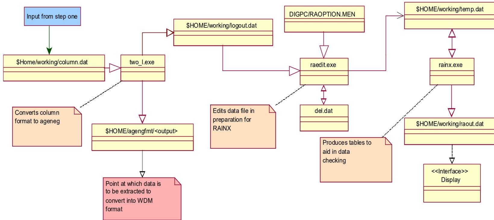
Figure 2.2 Data error checking, step 2.
