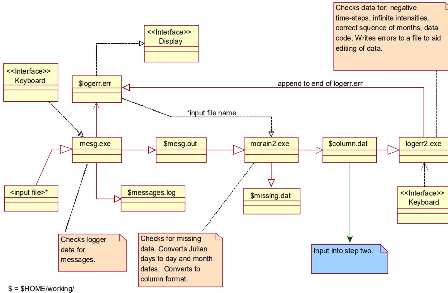
Figure 2.1 Data error checking, step 1.
