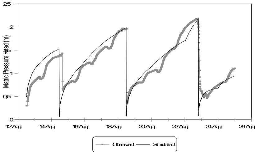
Figure 4.10a. Simulated versus observed matric pressure head at 0.19 m at nest 2, Willowfontein.
