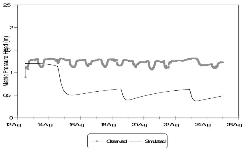
Figure 4.10b. Simulated versus observed matric pressure head at 0.72 m at nest 2, Willowfontein.
