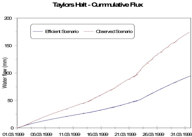
Figure 4.13 Comparison of simulated cumulative flow below the root zone for the observed irrigation strategy and a proposed efficient strategy for nest 1 at Taylor's Halt.
