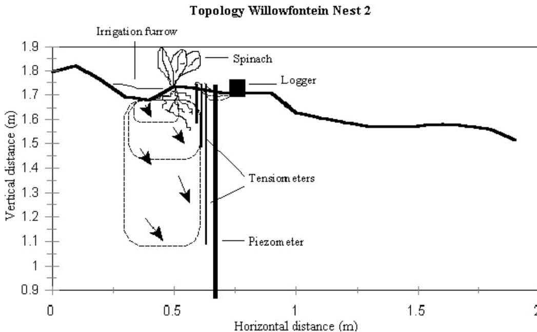
Figure 4.3 Ground surface topology at the Willowfontein, furrow irrigation site, showing a cross section of instrumentation installation, typical of both irrigation gardens.
