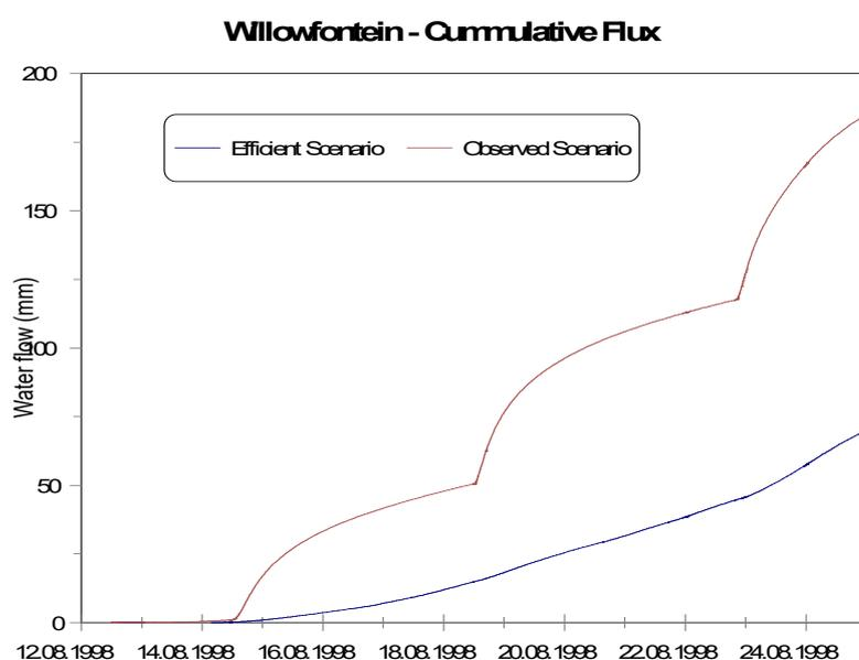
Figure 4.11 Comparison of simulated cumulative flow below the root zone for the observed irrigation strategy and a proposed efficient strategy for nest 2 at Willowfontein.
