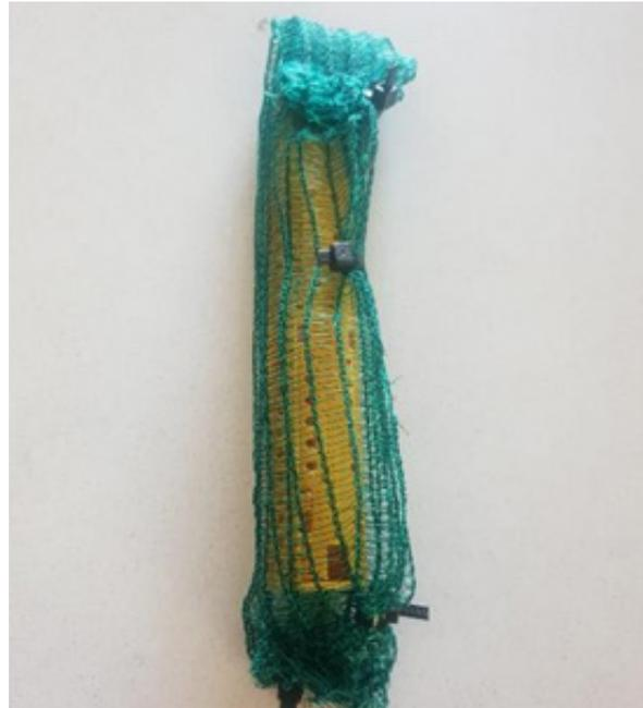
Figure 2. Passive sampling devices adapted for sampling non-sewered settlements
