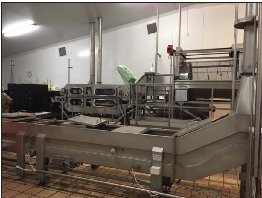
Figure 5.6: Industrial raw material washing at industrial unit 3013.9
