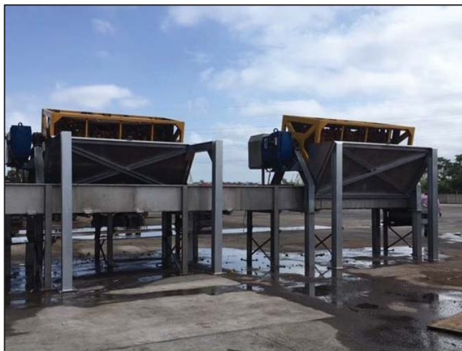
Figure 5.7: Facility 3013.12 removed the 'dumper baths' and now loads fruit directly onto conveyor belts
