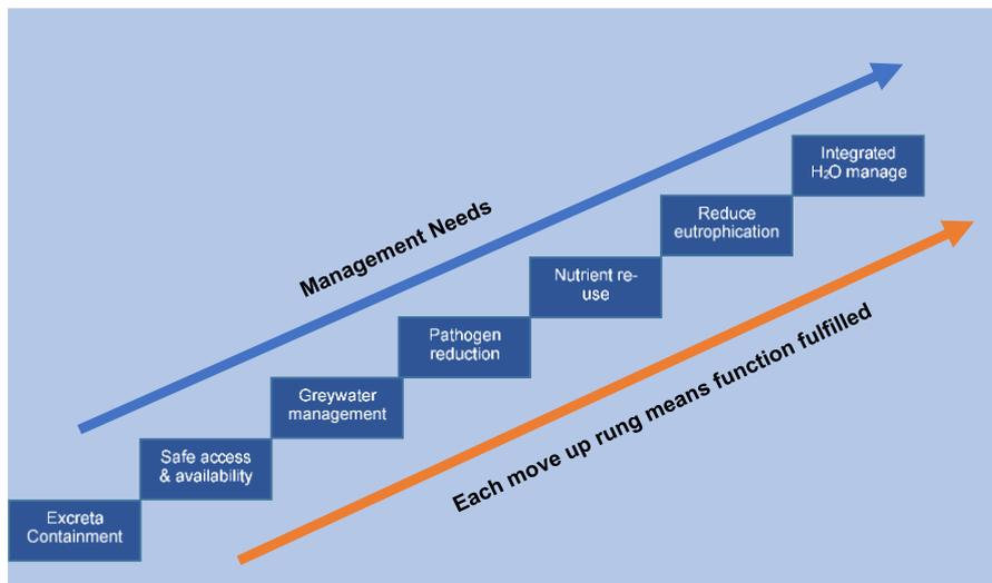
Figure 9. The Sanitation Ladder revamped from a technology-based approach to a function-based approach. Adopted from (Kvarnström, McConvilee, Brakcen, Johansson, & Fogde, 2011).
