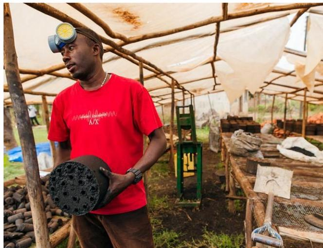
Figure 13. Briquettes made from collected and processed faecal sludge in Uganda.
