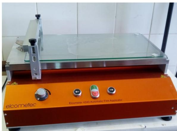
**Figure 8:** Casting membrane machine
