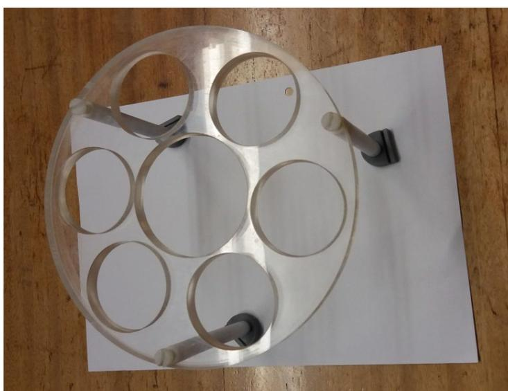
**Figure 15:** Passive sampler holder
