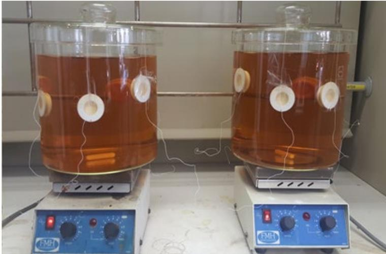
**Figure 26:** Experimental set up of SCPEI-PCPEI-based DGT sampling devices in AMD water.
