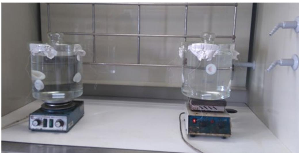
**Figure 22:** Laboratory-based deployment of passive samplers in Spiked Milli-Q water.
