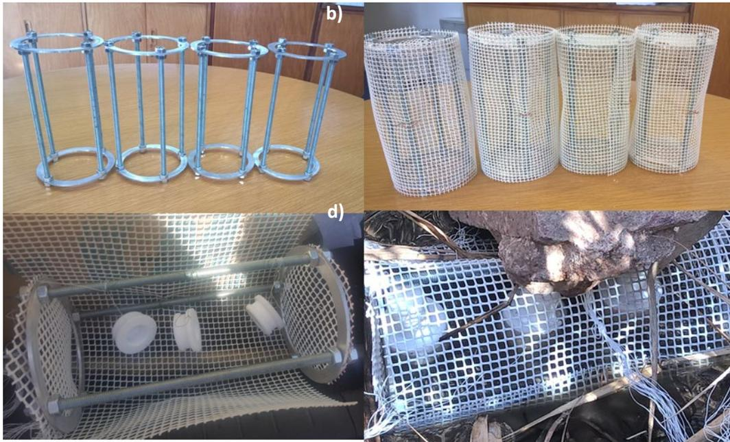
**Figure 23:** a) and b) Cages used for housing the passive samplers during field deployments, c) passive samplers attached to the sampling cage d) picture of passive samplers submerged in the field.
