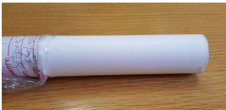
**Figure 20:** PTFE rod used in the construction of DGT sample holder units
