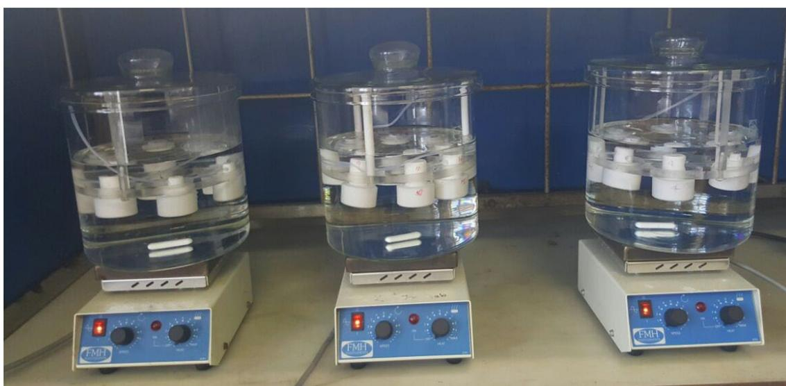
**Figure 16:** Set up for polymer inclusion membrane passive sampler
