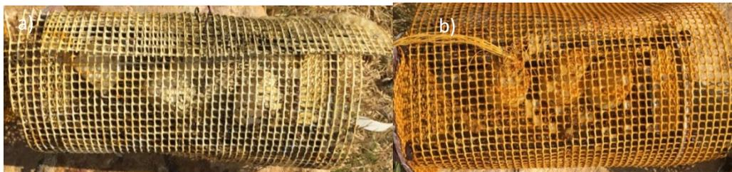
**Figure 59a:** Picture of PIM-based passive sampler cages after deployment of a) day 2 and b) day 12 at AMD
