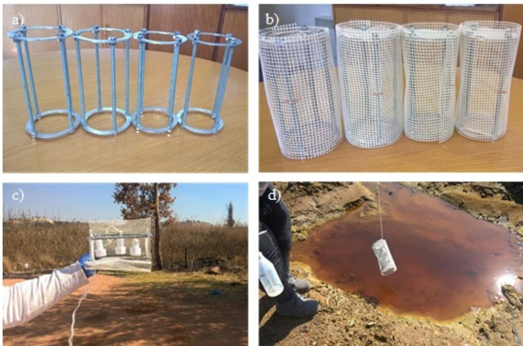
**Figure 19**a) threaded steel rods and b) plastic mesh was wrapped around the steel rod structure in order to seal the Cages used for housing the passive samplers during field deployments, c) and d) deployment of the passive samplers, (e) picture of passive samplers submerged in the field.
