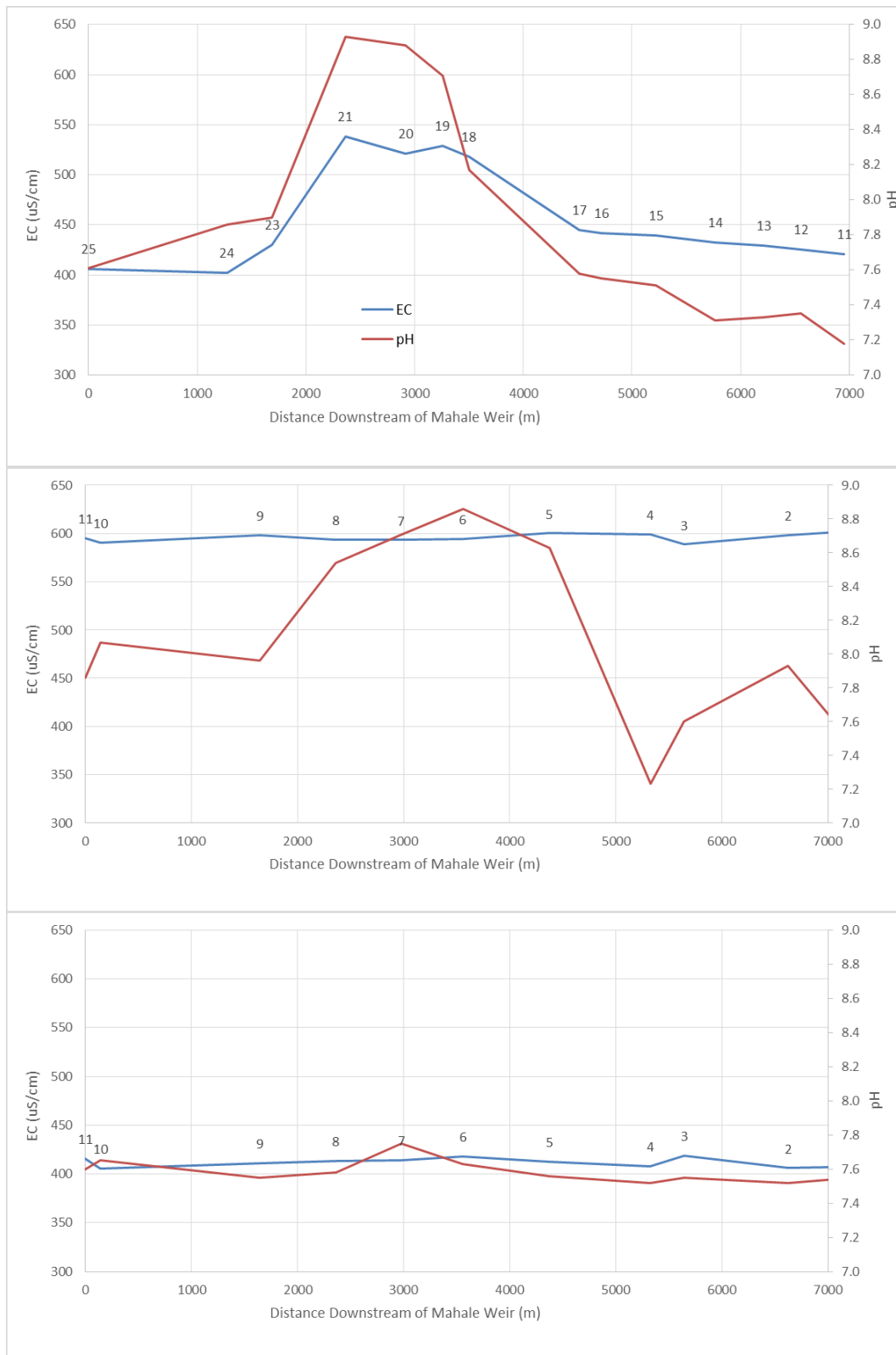
Figure 11: Longitudinal hydrochemical surveys of the Letaba River between Mahale and Letaba Ranch on 24 November 2014 (top) using in situ measurements on 27 October 2015 (middle) and 14 April 2016 (bottom) using samples analysed by the MOSA Mobile Laboratory 5
