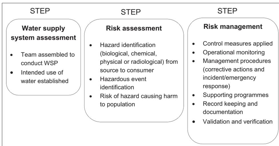
**Figure 4-1: Steps to assess water supply based on the WSP approach (Source: Thompson and Majam, 2009)**
