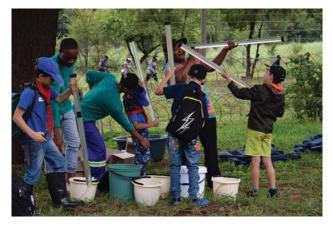
Hlengiwe Cele from the WRC demonstrates how to use a clarity tube to assess turbidity – an indicator of water quality.
