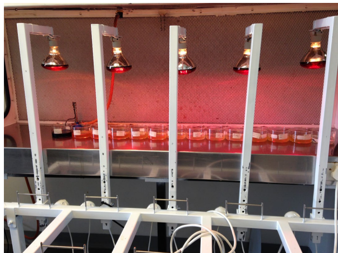
Figure 7. Set up of the micro scale evaporation rate experiment.
