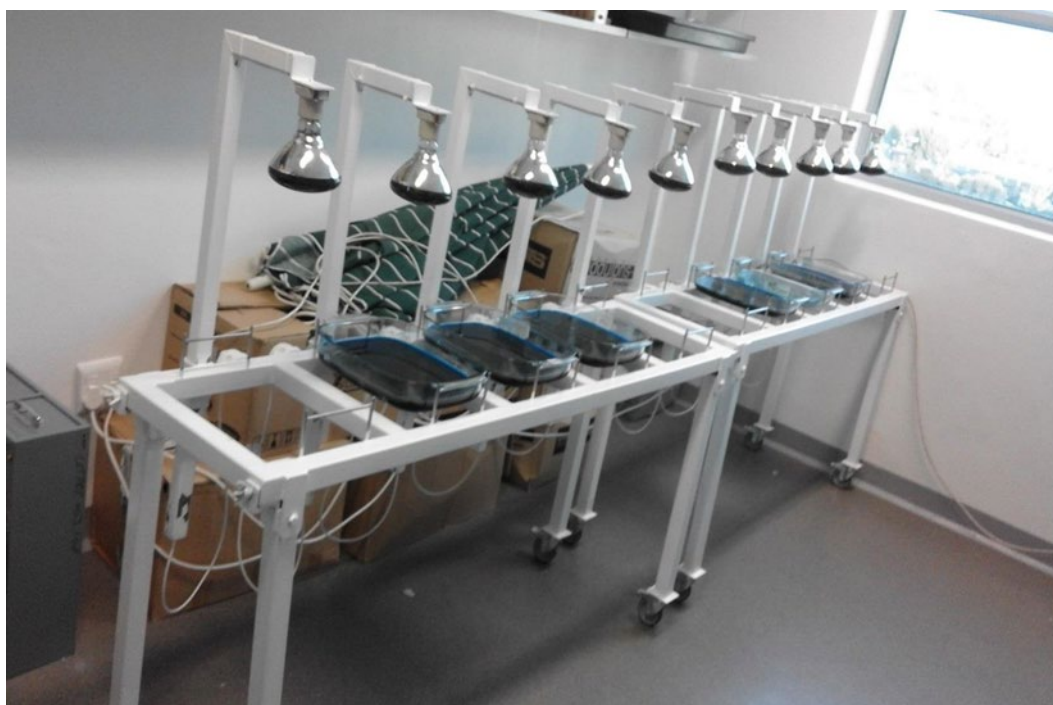
Figure 6. Experimental set up for methylene blue evaporation studies.
