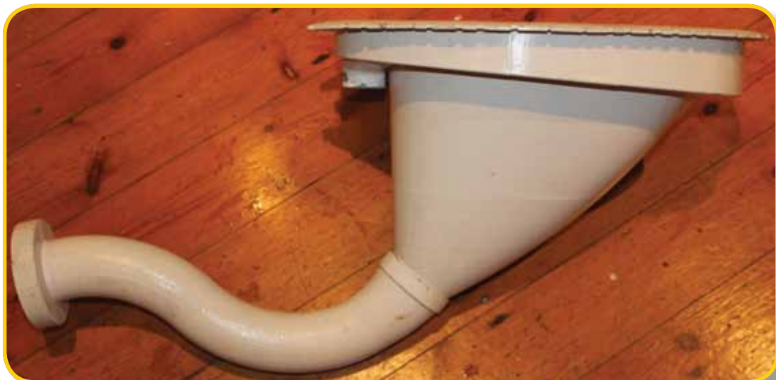
Prototype pan and gooseneck outlet
