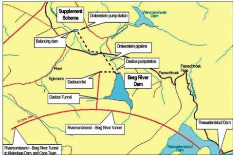
The Berg Water Project comprises the Berg River Dam (which is about 6 km west of Franschhoek) and the Supplement Scheme situated about 12 km downstream. The latter comprises a 1,6 m-high diversion weir that diverts a portion of the winter high flows into a 3 ha off-channel balancing dam from where the water is pumped via a 12 km pipeline back into the Berg River Dam.
