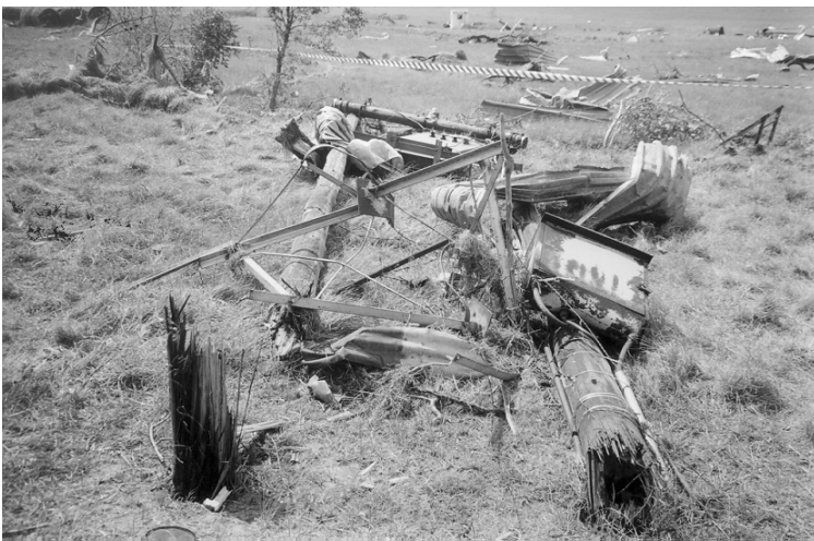
Figure 5 Remains of a telephone line (Goliger and Van Wyk, 1999)
