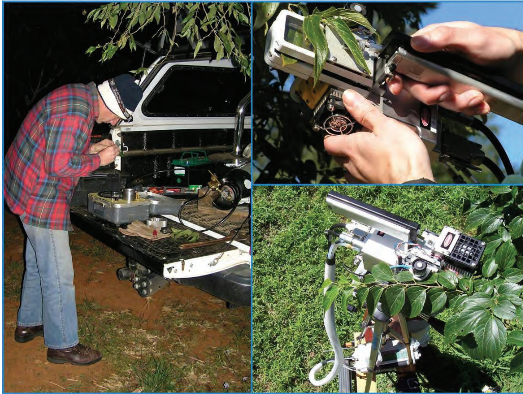
Figure 9.10 Measurements of pre-dawn xylem pressure potential (left) and photosynthesis using a “SunSky” chamber (right, top) and a RedBlue chamber (right, bottom).
