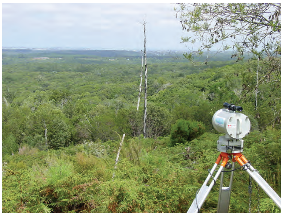
Figure 3.7 The LAS transmitter positioned on the upper edge of Groenkop forest and pointing towards the LAS receiver in the distant building (Research block, North campus).
