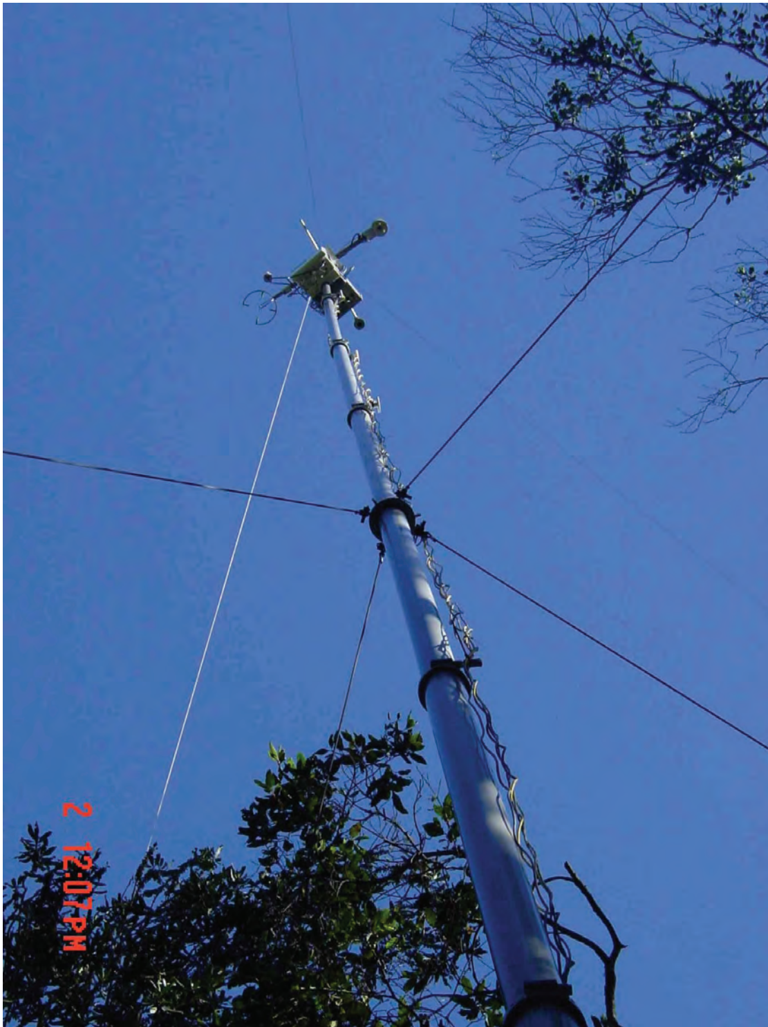
Figure 3.4 The fully extended mast showing supporting stays and instruments mounted on a cross-arm near the top.
