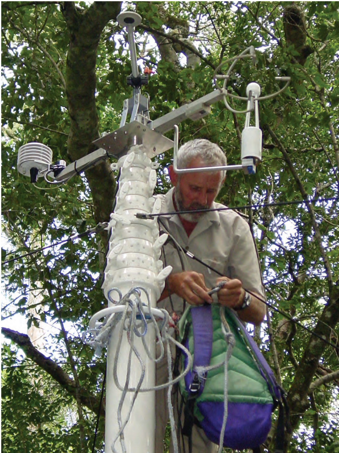
Figure 3.3 The Eddy Covariance sensors attached to the top of the telescopic mast.
