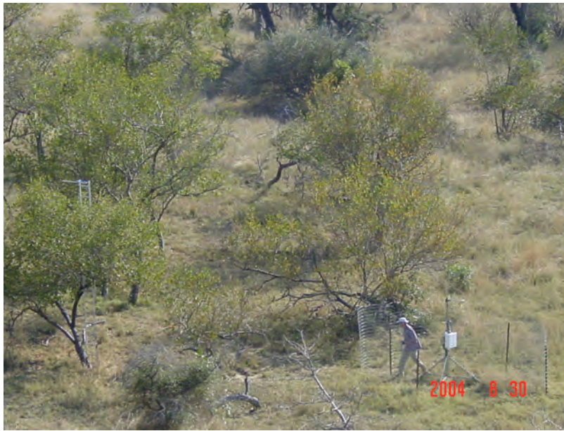
Figure 5.4 View of the net radiation sensors located over grassland and over a Combretum tree canopy. Soil heat flux was also measured under grass and under trees.
