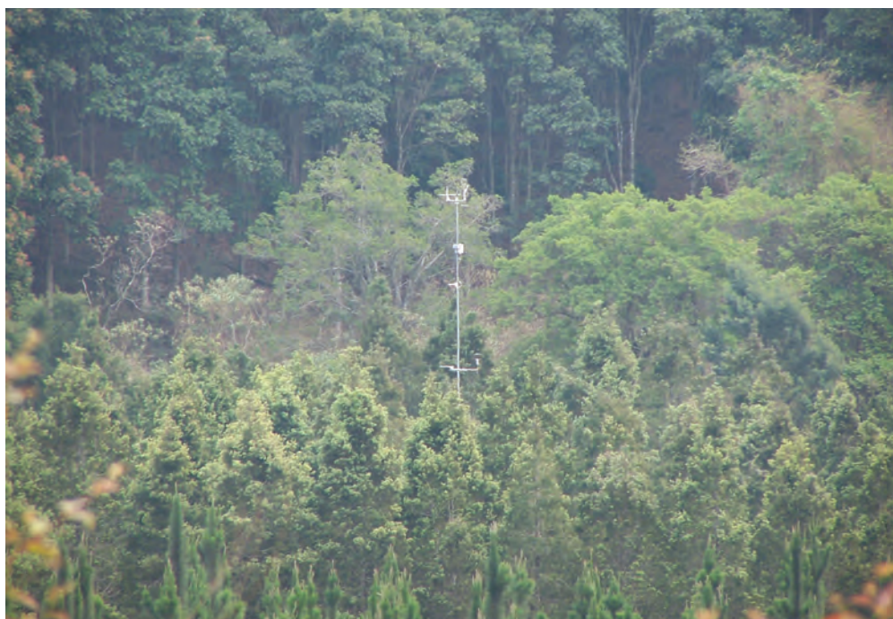
Figure 4.1 A view of the instrument mast and sensors positioned above the Podocarpus falcatus tree canopy at the Magoebaskloof site.
