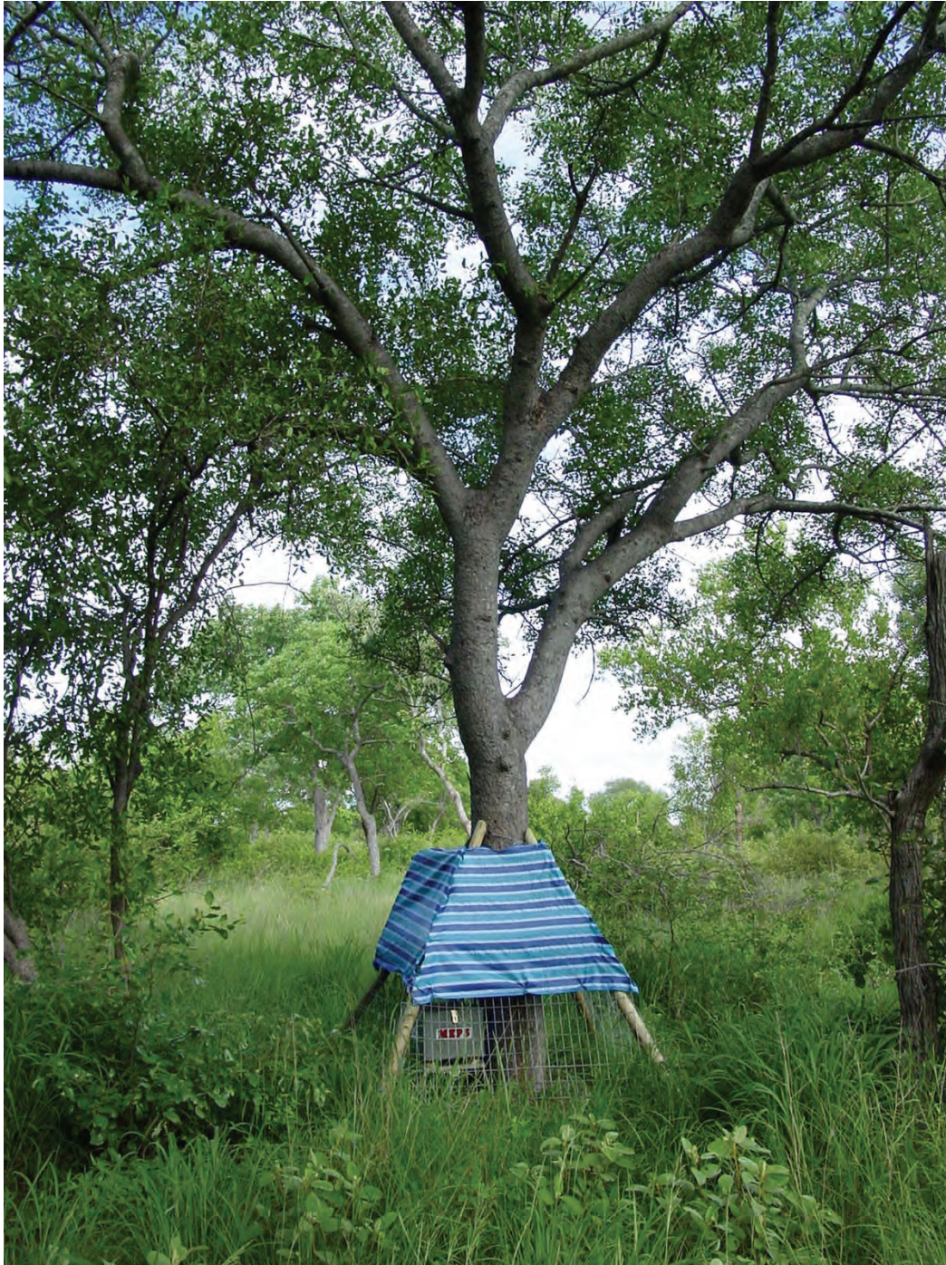
Figure 5.9 A sample tree showing the weld mesh enclosure and shade cloth awning used to protect the heat pulse equipment. The vegetation depicts the green conditions that existed during the February 2004 visit.
