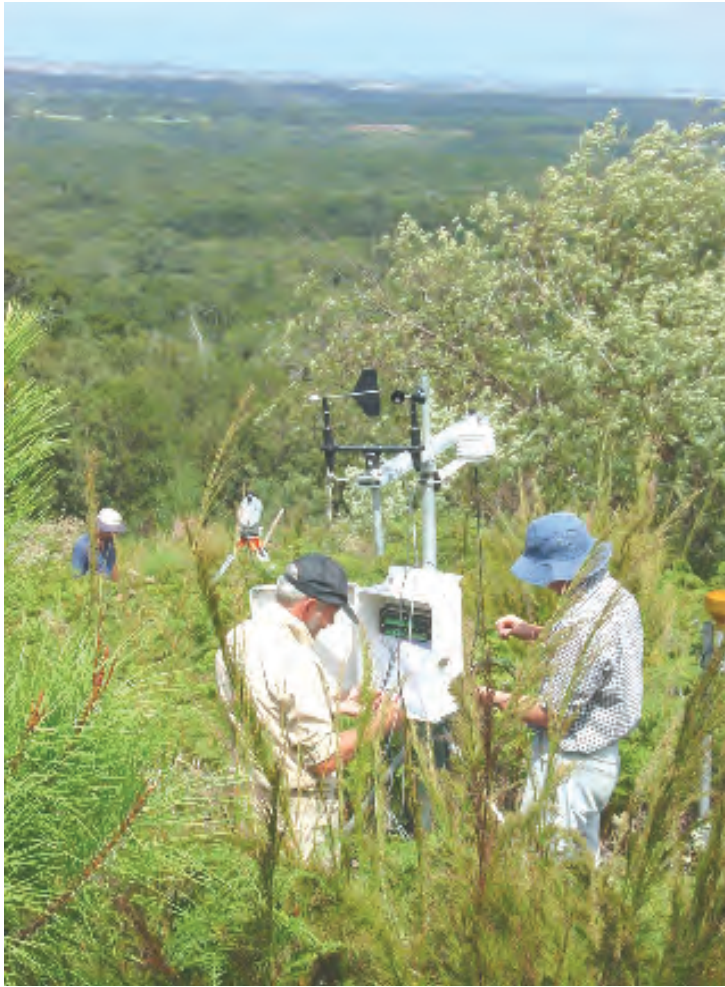
Figure 3.8 An automatic weather station erected behind the LAS transmitter on the edge of the Groenkop forest.
