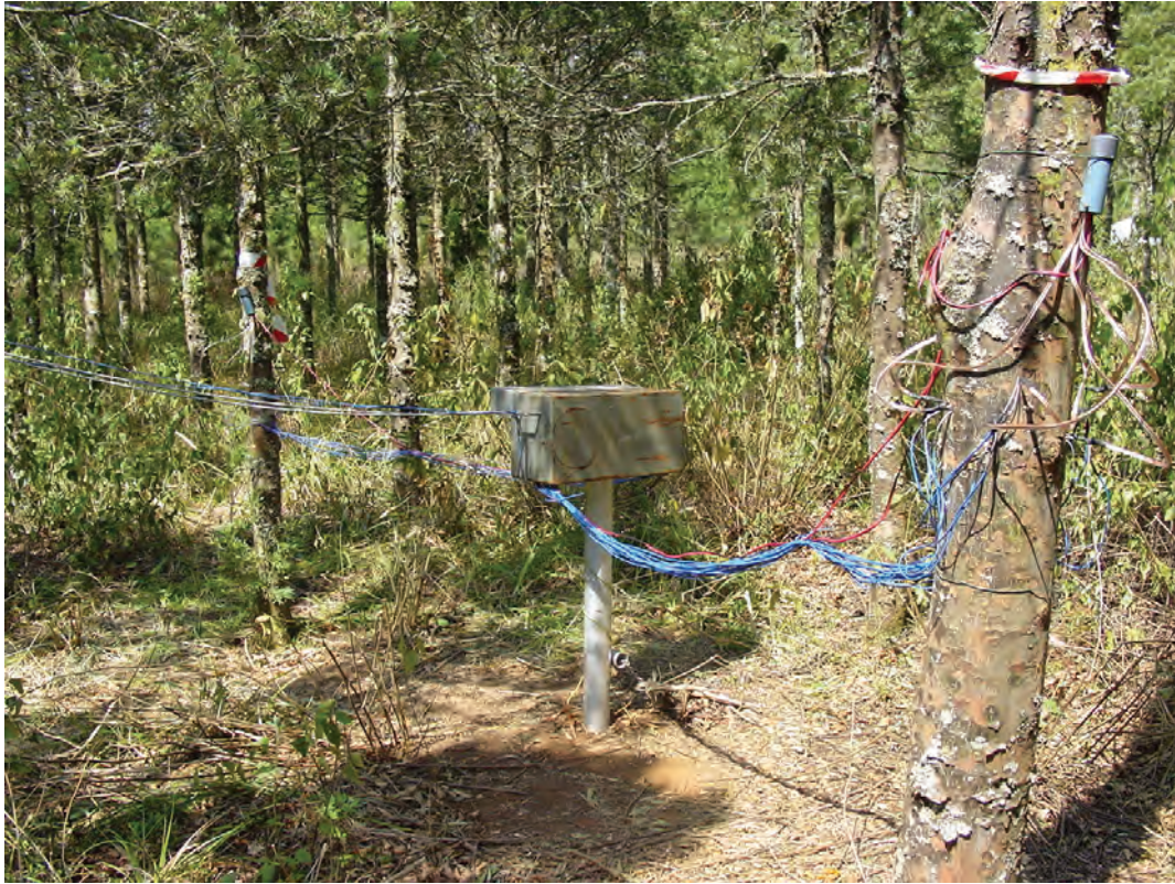
Figure 4.4 A view of one of two heat pulse velocity systems used to monitor sap flow rates in a sample of Podocarpus falcatus trees at the Magoebaskloof site.
