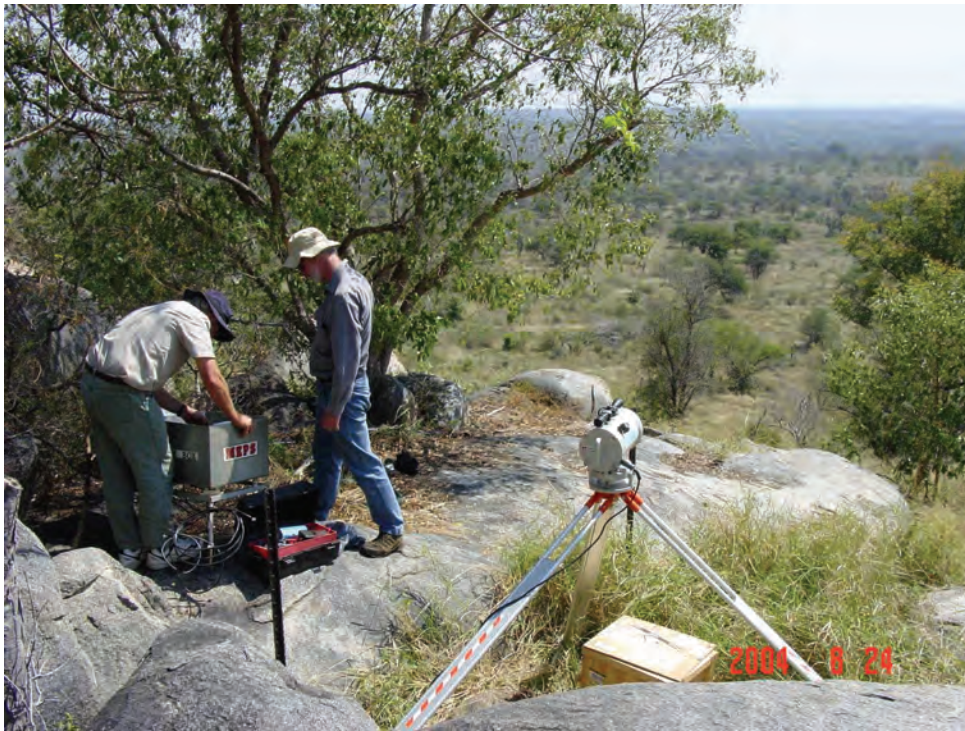
Figure 5.1 The LAS scintillometer transmitter deployed in the Kruger National Park.
