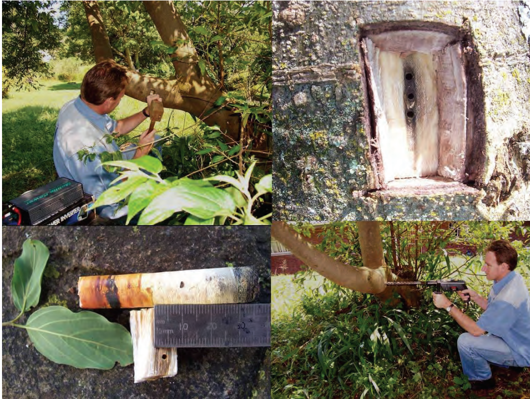
Figure 9.7 Collection of wood samples to determine sapwood properties required for final HPV calculations.
