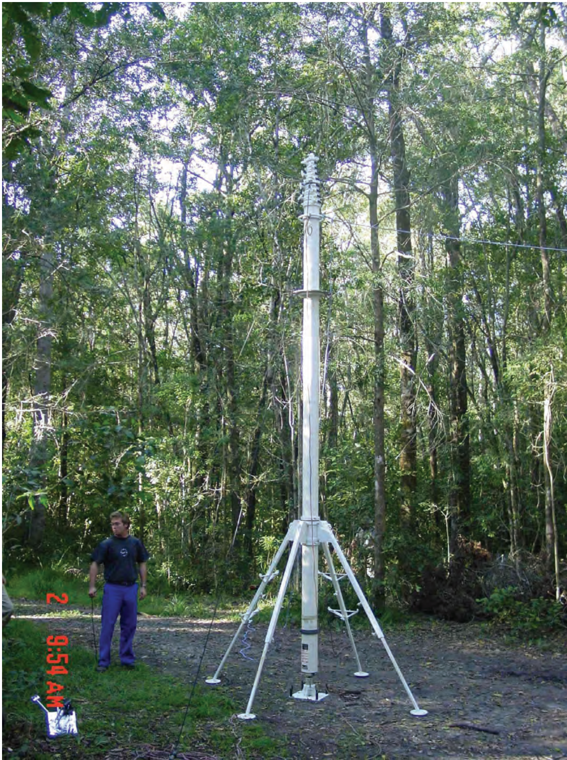
Figure 3.2 The telescopic mast ready for extension to its full height.
