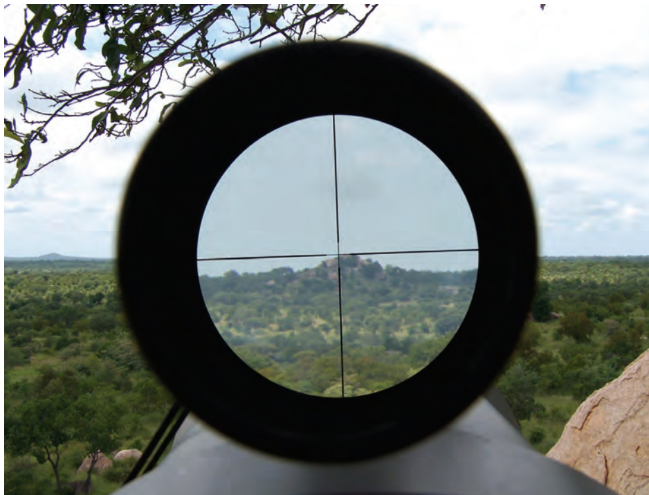
Figure 5.2 A view through the scintillometer sighting scope along the beam path to the transmitter station.
