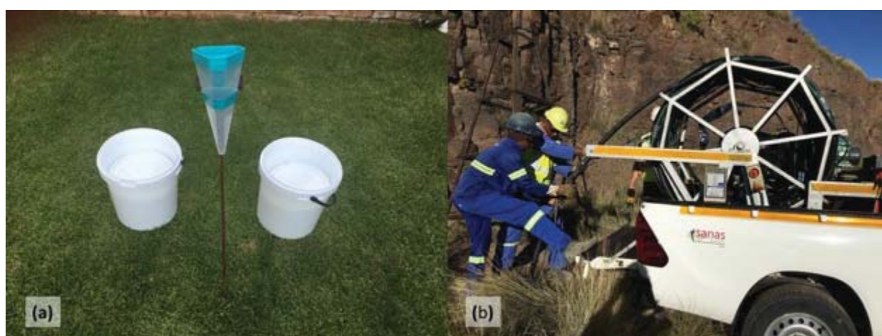
Figure 9-6. Sampling: (a) rain gauge and 20 litre water buckets for rainwater sampling; (b) purging of GWF12 (VZSA09).
