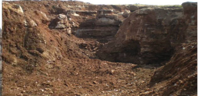
(c) Sinkhole in Khutsong; shallow dolomite with dissolution features, interlayered with chert (3 May 2018).
