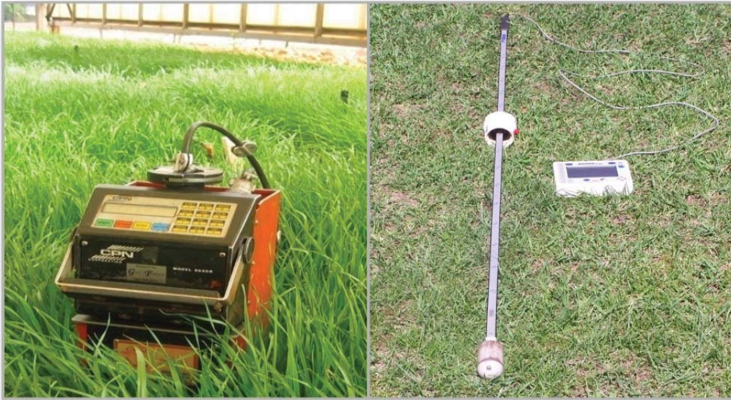
Figure 2.1 A neutron water meter (left) and Diviner 2000 capacitance probe (right) for measuring soil water content
