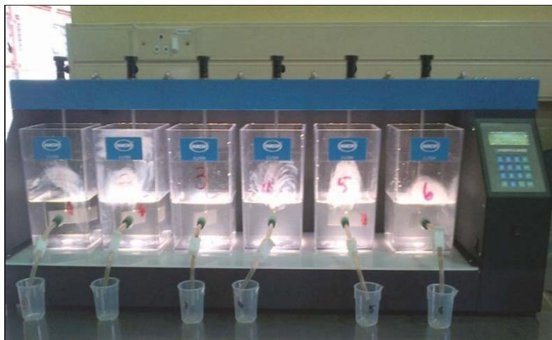
Figure 7.1: Jar test equipment set-up
