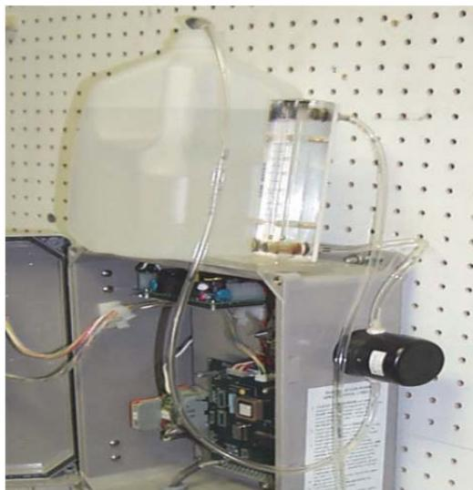
3. To hook up the tubing as shown in the picture, you will need one 3 foot piece of tubing going from inside the jug to the bottom of the sensor (Note: Rinse off tubing with clean water before inserting into the jug). Next is an 8 inch piece of tubing going from the top of the sensor to the bottom fitting of the rotameter. Finally, there is a 4 foot piece of tubing that is connected to the top fitting of the rotameter. Install the tubing clamp on the 4 foot piece of tubing.
