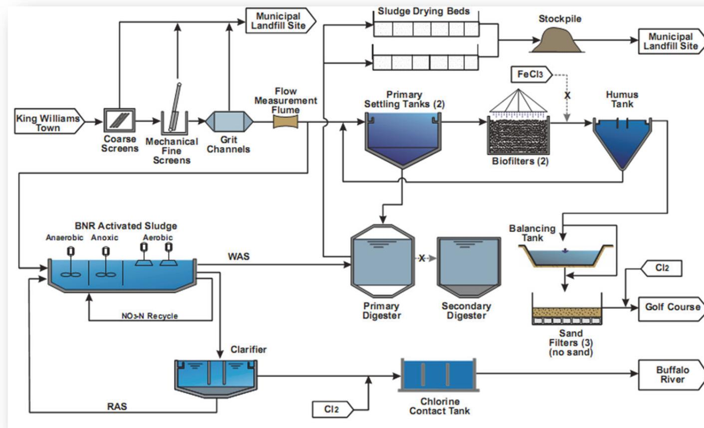
**Figure 1:** Combined trickling filter and activated sludge process with sludge drying beds and stockpiling for sludge management, example of a system flow diagram completed from selecting the icons on the previous pages.
