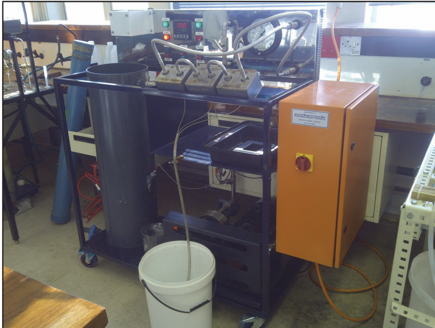
Figure 3.8: Membrane Test Unit
