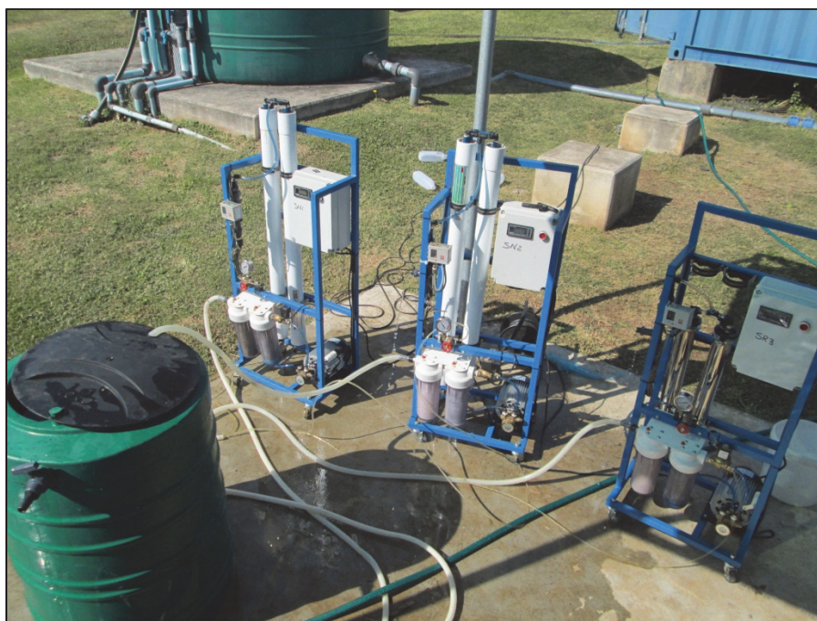
Figure 3.10: RO Membrane Test Rigs Operating in Parallel
