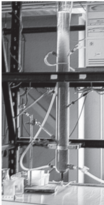
Figure 51: Aerobic Granular Sludge laboratory reactor setup (photo from de Kreuk PhD thesis, TU Delft 2006)
