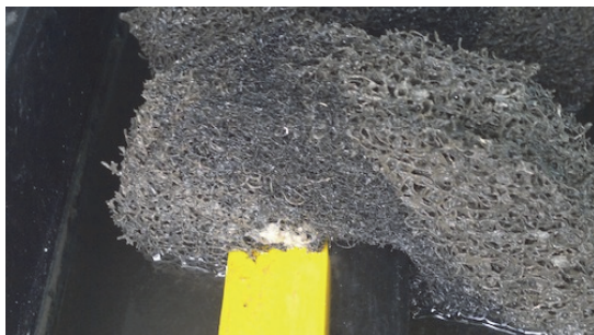
Figure 79: Biofilm growth on mesh causing imbalance on disk – a common problem in earlier RBC designs globally.
