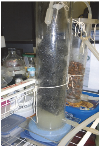
Figure 80: A trickle bed reactor with two support media alternatives, inoculated with synthetic media and Isolate 1: To the left is the mesh used in the RBC, and to the right is a lightweight expanded clay aggregate ('LECA balls').
