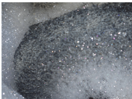
Figure 63: Close-up: Growth of biofilm on mesh of rotating biological contactor.
