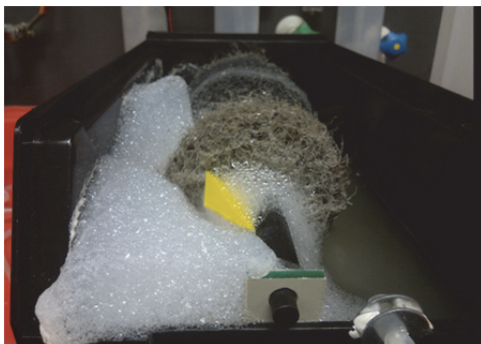
Figure 62: Growth of biofilm on mesh of rotating biological contactor.
