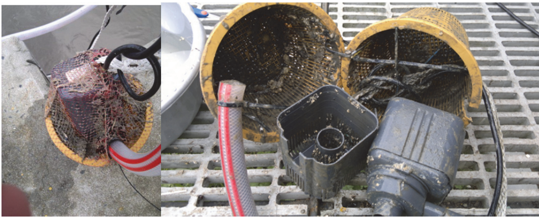
Figure 85: Fishpond filter covered in grease and particulates. The white crumbs are either grease or polystyrene particles.
