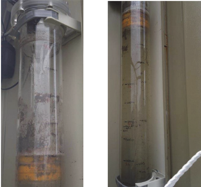
Figure 67: First days after start-up: The AGS reactor with raw sewage and granules looking possible.
