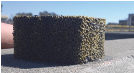
Figure 83: Fishpond filter foam covered in grease and particulates.
