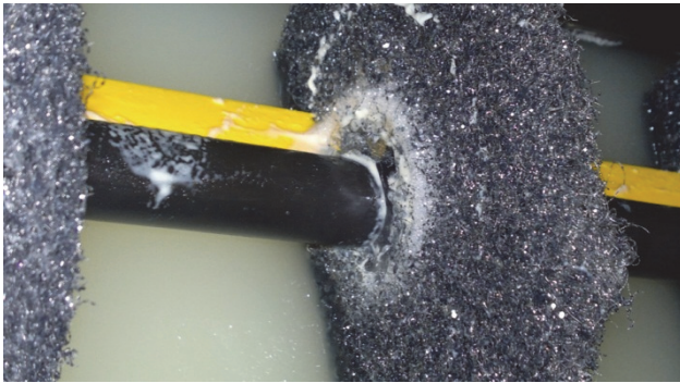
Figure 65: Close-up: Growth of biofilm on mesh of rotating biological contactor with more dilute substrate feed. Note that much of the biomass is still in the liquid phase.
