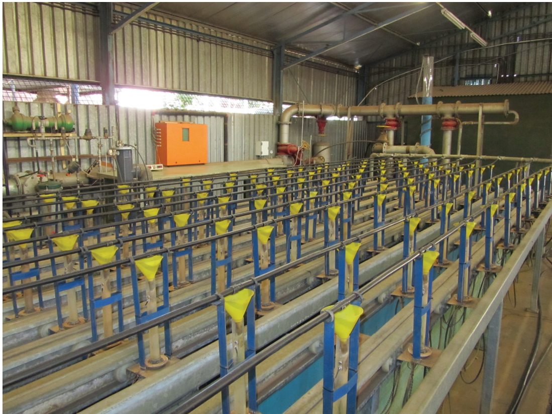
Figure 4: Test bench for emitter discharge and CV_q tests
