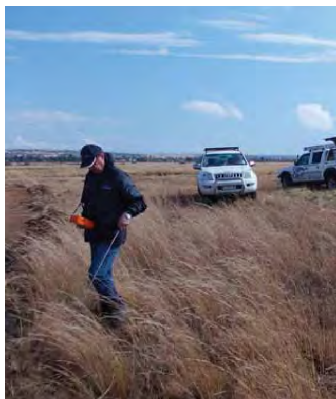
Figure 1: Physically walking a pipeline route to detect leaks using leak detection equipment
