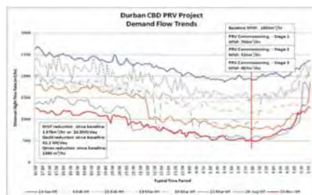
Figure 3: Changes in flow profile into Durban CBD at various stages of PRV commissioning
