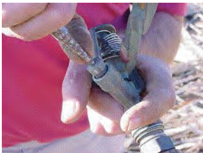
Figure A1.6: Measuring apparatus for sprinkler nozzle size
