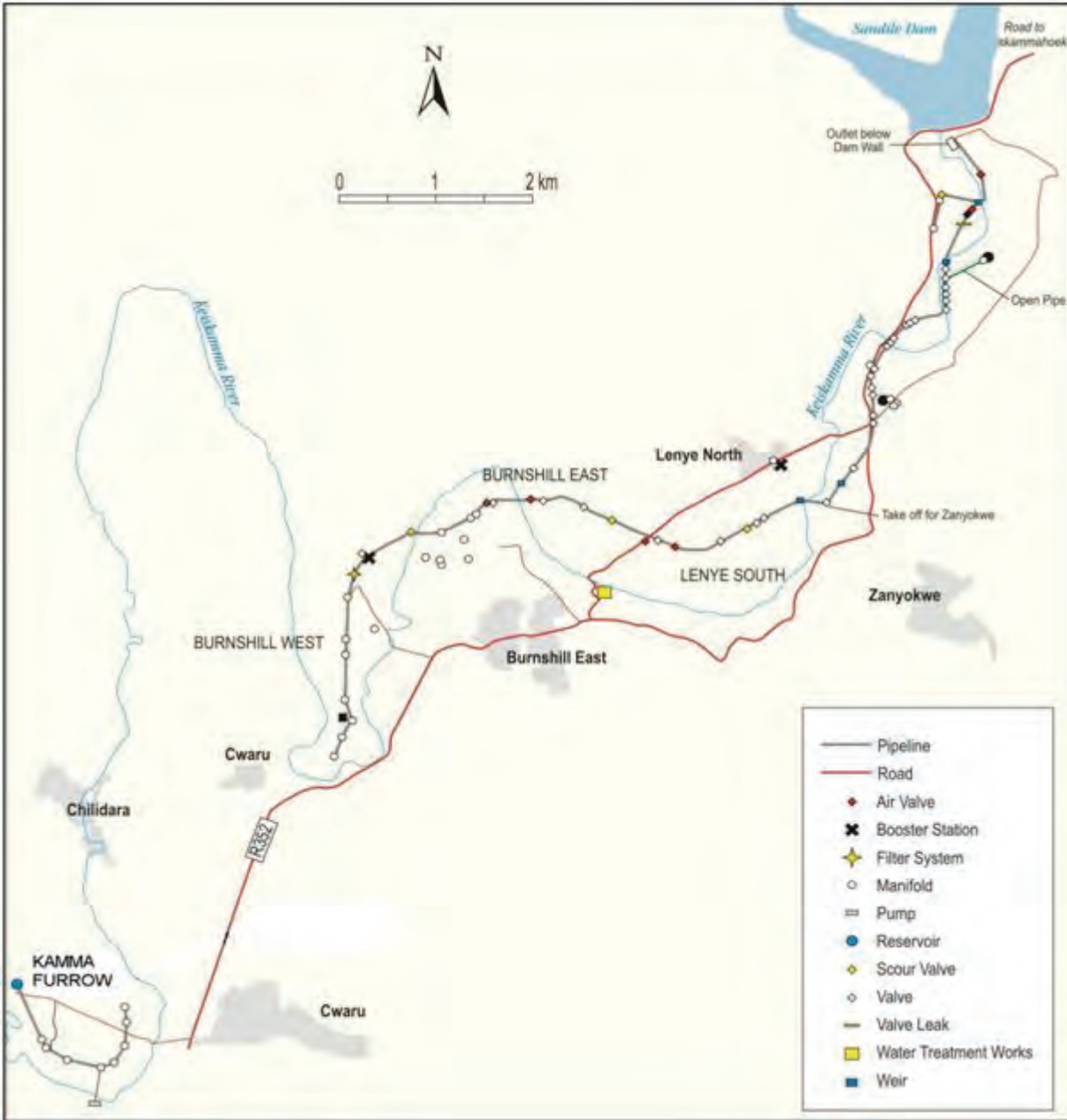
Figure 2.1: Schematic diagram of the Zanyokwe Irrigation Scheme
