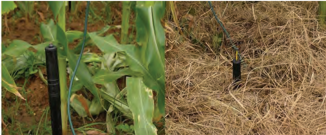
Plate 3.14: Wetting front detectors (15 cm deep) generally indicated low soil water content where no mulch was applied (left) compared with mulch treatment (right).
