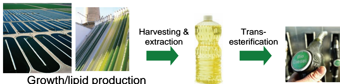
Figure 3: Growth of algae for the production of biodiesel
