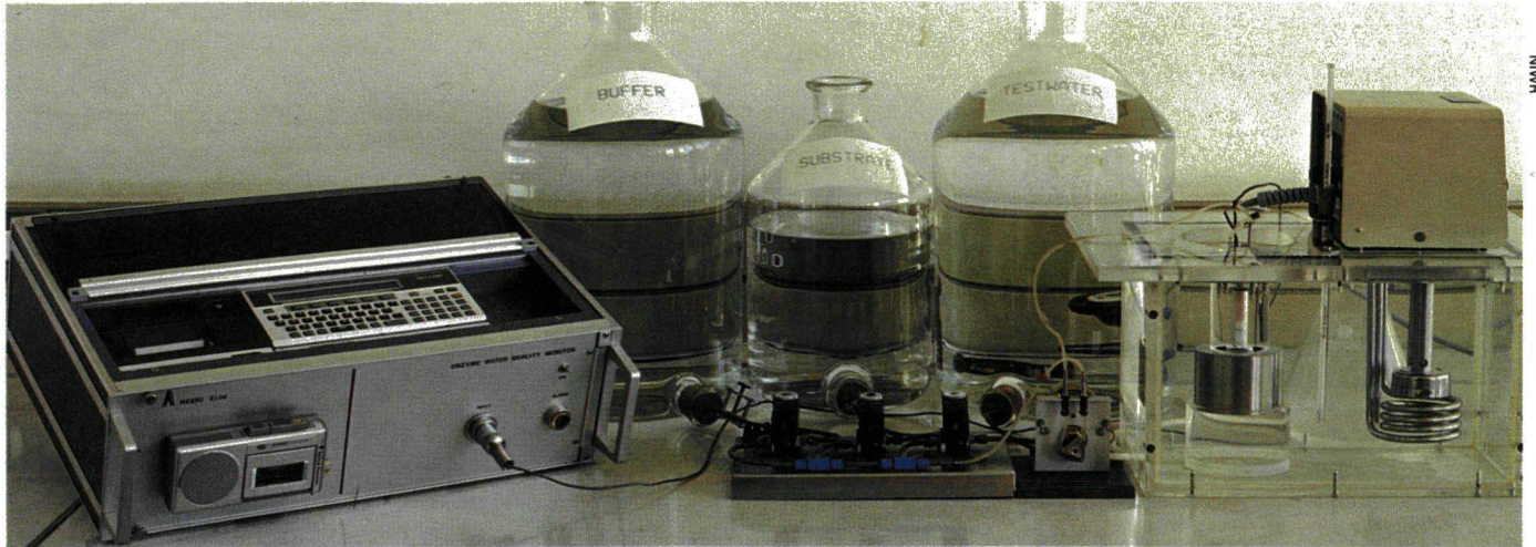
An enzyme microcalorimeter is used in the continuous automatic enzyme monitoring system. This system is R20 000 cheaper than a biological monitoring system.
