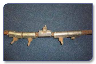
Figure 12: A case where pipe replacement is clearly appropriate
