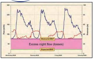
Figure 8: Example of a basic flow and pressure logging
