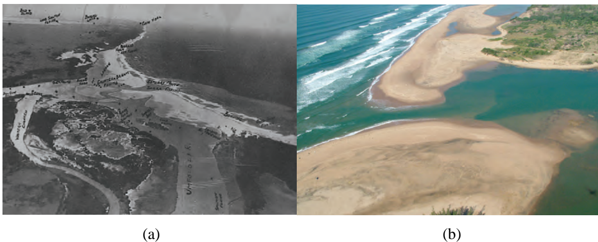
Figure 7. (a) A combined St Lucia and Mfolozi system, illustrating the complex dynamics at the estuary inlet and the formation of flood deltas. (b) An artificially separated St Lucia mouth configuration illustrating the spit migration due to long shore transport and the formation of a flood delta due to the influx of sediment into the estuary (pictures courtesy of R. Taylor).
