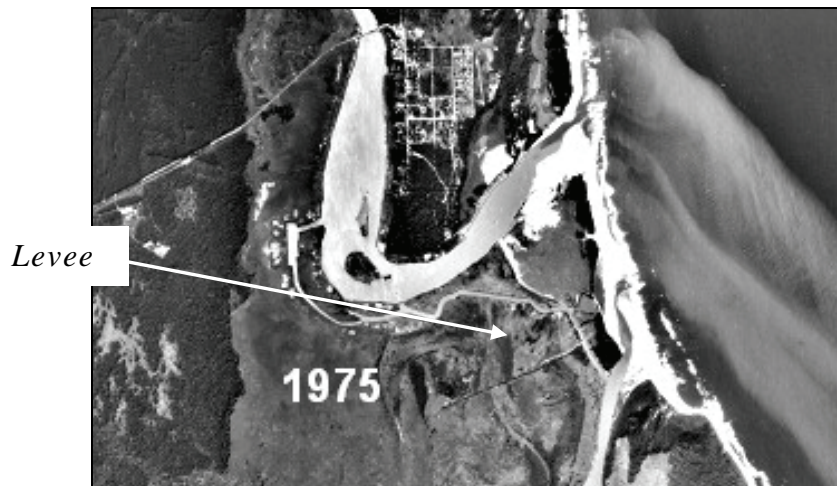
Figure 11. Aerial photograph (1975) showing the position of the “Back Channel” south of the St Lucia Estuary and linking through to the Mfolozi Estuary. Also visible is the levee from ENE to WSW that was excavated to prevent the sheet-flow of floodwaters from the Mfolozi towards St Lucia.
