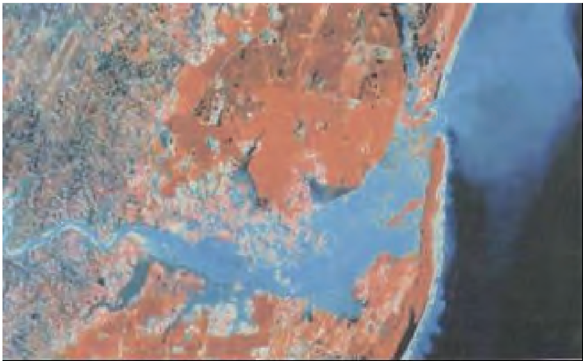
Figure 4. LANDSAT image (NASA) from the 1987 flood showing the full extent of the inundated floodplain. This floodwater delineates the margins of the floodplain and is used in subsequent illustrations.
