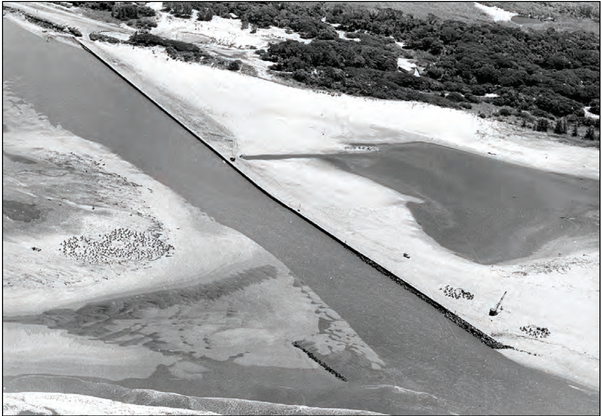
Figure 10. Aerial photograph of the St Lucia mouth taken in about 1974, showing the groyne built to stabilise and constrict the mouth. The north groyne was built first followed by the smaller one on the south bank. The estuary mouth is at the lower right corner of the picture (photograph: R. Taylor).
