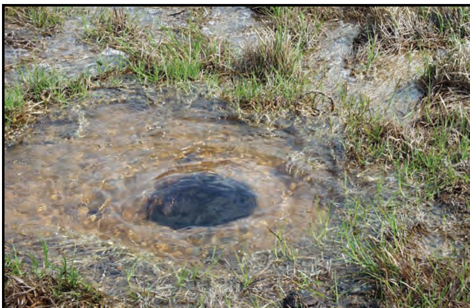
Figure 9.1: The first water to decant from the flooded mine void occurred from a borehole sunk into a dolomitic inlier which, in turn, is linked to flooded mine workings. This borehole is next to the Tweelopiespruit (photo: G. Krige, 28 August, 2002).
