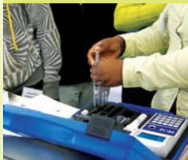
A mini-lab kit allows staff to do on-site testing for pH, nitrates, ammonia, ortho-phosphate and MLSS.
