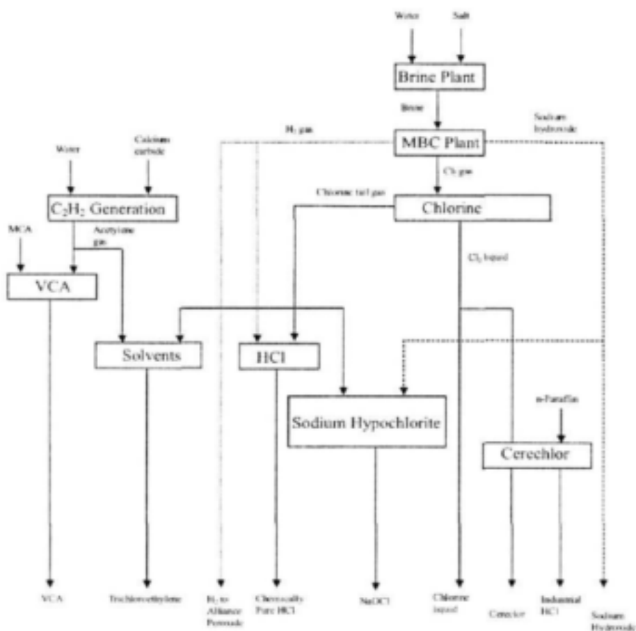
Figure 4.1: The chlor-alkali and related processes at the Sasol Polymers plant, Umbogintwini.
