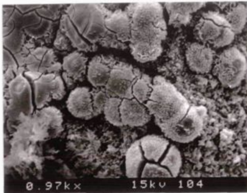
Figure 5: Corrosion product and crystals on the MS coupon surface.
