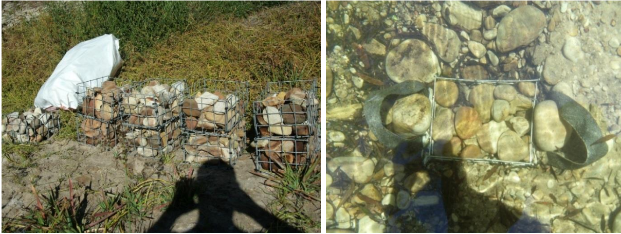
Figure 5: Sediment Infiltration baskets filled with gravel used in capturing fine sediment (left); embedded basket in riverbed (right)
