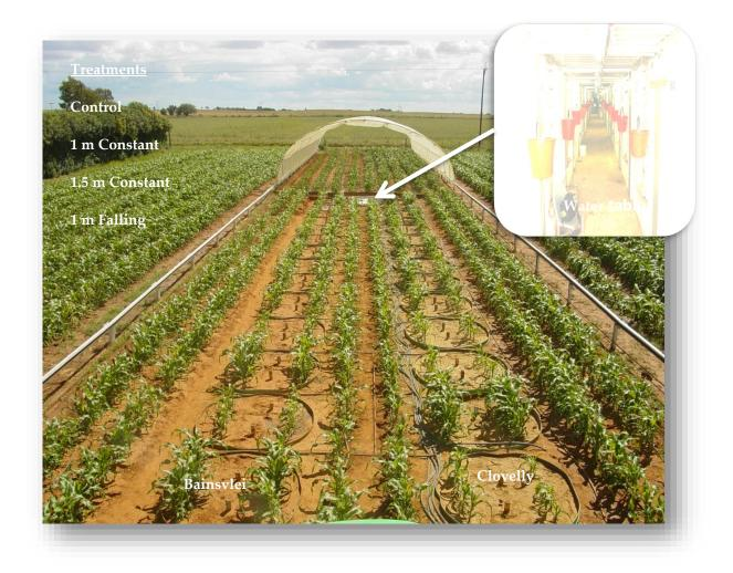
Figure 10.3: Lysimeter trial for evaluation of different groundwater levels.
