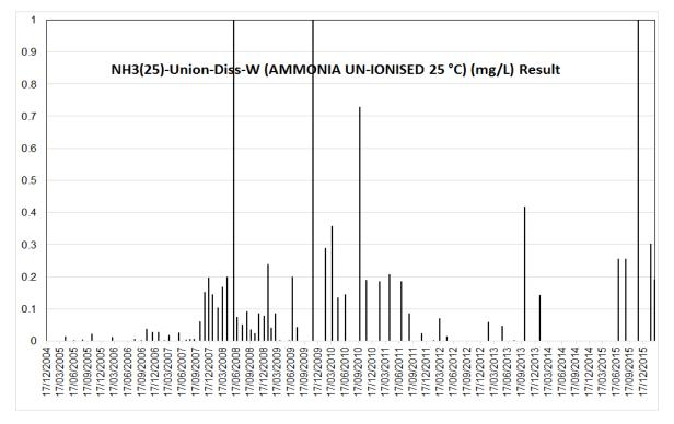
Figure 15: Records of readings for un-ionised ammonia (NH3) concentrations at gauge 200000109, Kuils River
