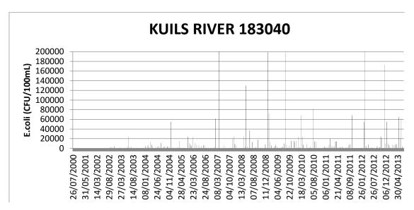
Figure 16: Record of E.coli counts in Kuils River at Zandvliet Bridge downstream of Zandvliet sewage works
