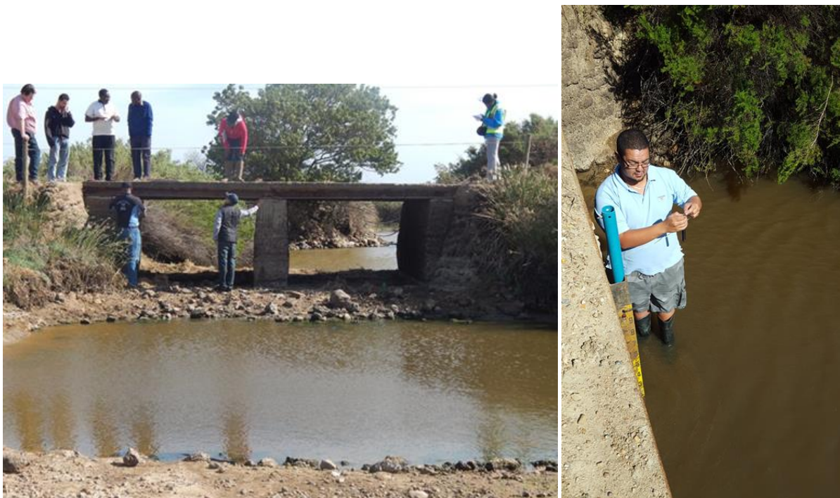
(b) Nuwejaars River at Elandsdrift flow measuring station, and, on the right, Daniel Mehl (MSc student) retrieving a data logger from the blue PVC which acts as a stilling well.
