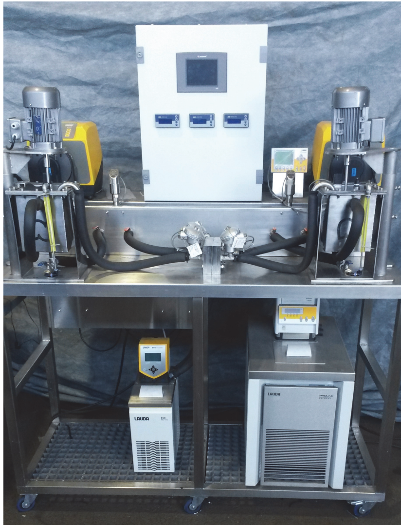
Figure 28: Photograph of commissioned DCMD experimental set up
