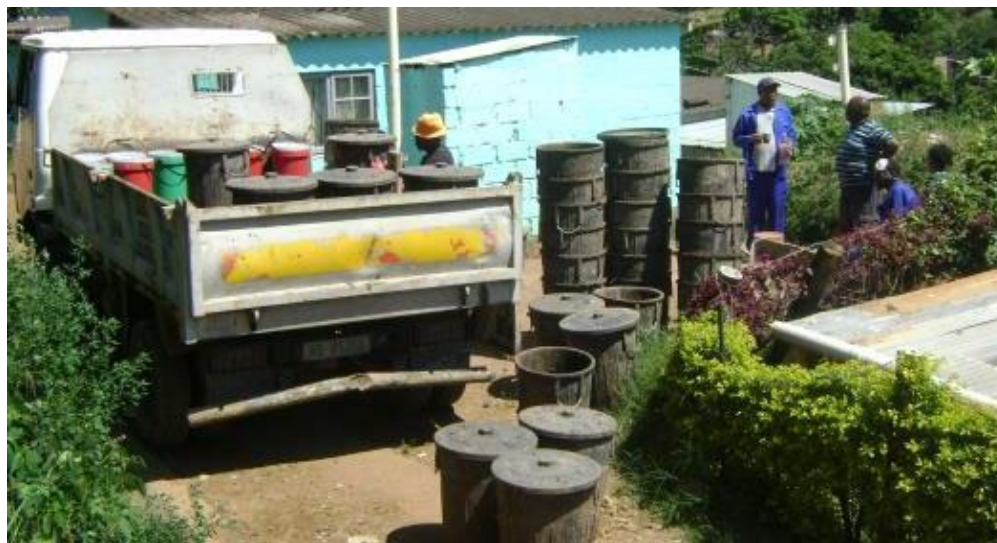
Figure 33: A vehicle from a local hardware was hired to transport the bins to the disposal site. Several people from the community passed through the area where sludge was being loaded or empty bins off loaded. The vehicle was contaminated by the workers' gloves, boots and the bins.
