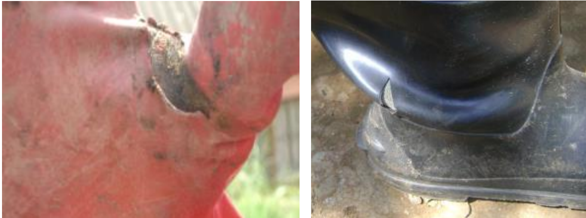
Figure 10: A torn glove (left) and boot (right) which no longer provide an effective barrier.
