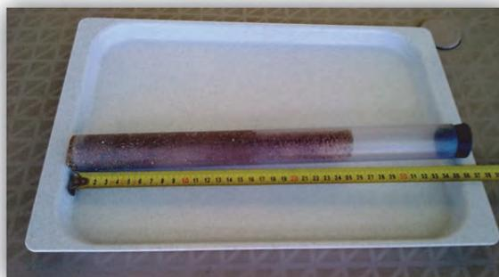
Figure 3: Perspex corer with core sand samples extracted from a biological sand filter
