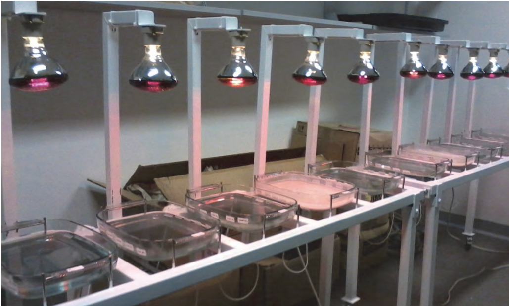
Figure 3.3: Experimental set-up for brine evaporation in shallow basins mounted beneath infrared lamps with adjustable height
