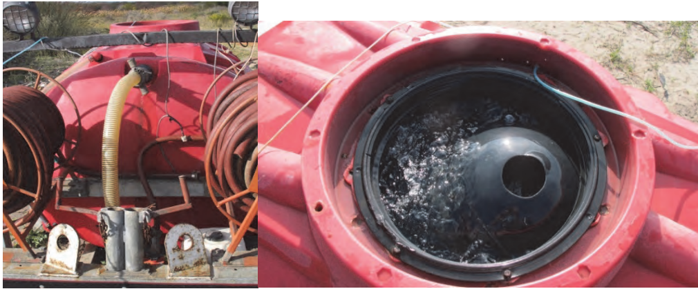
Figure 44: The water in the tank was further aerated by running the motor-driven pump where water was drawn from the base outlet through the yellow pipe (left) to the top outlet, which increased the exposure to the atmosphere (right)
