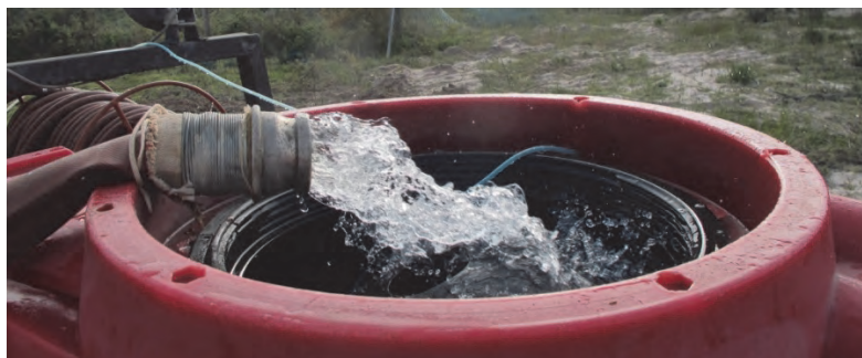
Figure 43: Aeration of the abstracted water from G30966 was achieved by splashing the water onto the baffle balls as it entered the water tank
