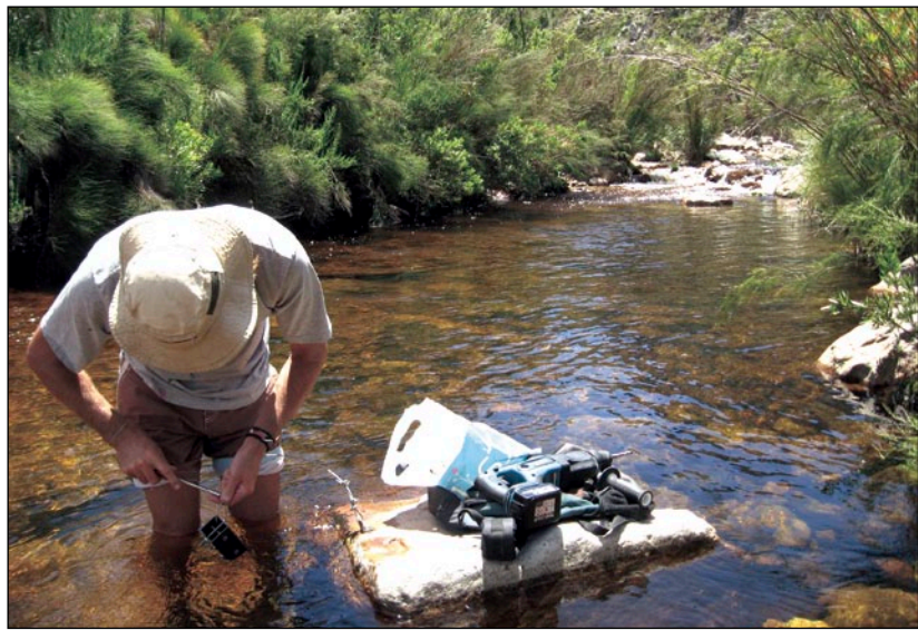
The water temperature loggers are secured via steel cabling onto a bolt drilled into rocks in the river channel. Here Cameron Dallas displays some brotherly love by doing manual labour for his sister's project.
