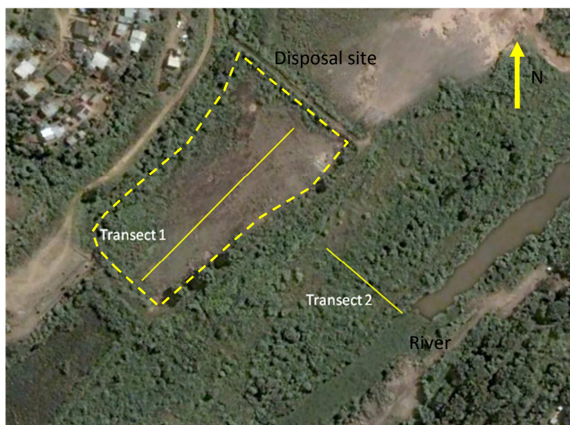
Figure 5.7 Transects used for ERT survey in September 2008
