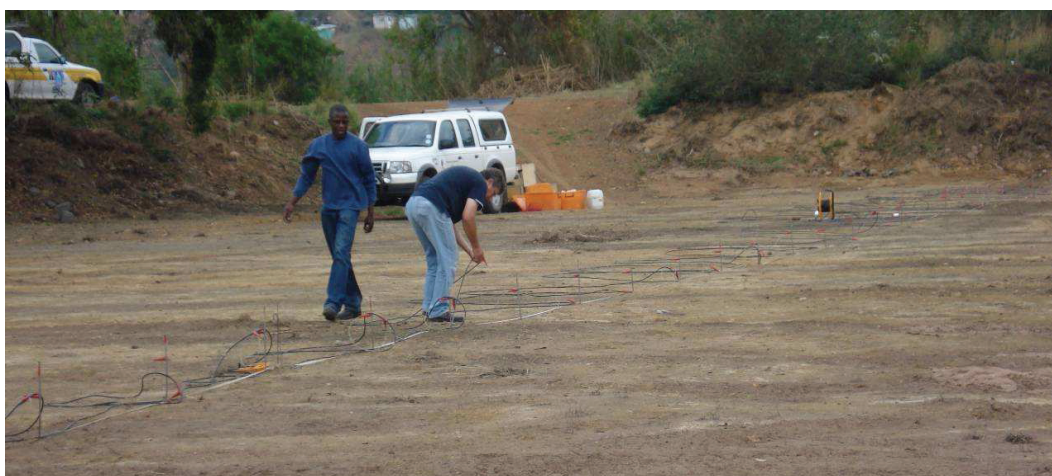
Figure 5.4 ERT survey at Umlazi to determine subsurface layering and soil water profile
