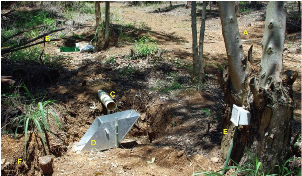
Figure 3.18. Water from the stilling well is directed to the tipping bucket. A Hobo event logger records the number of tips. A: lower gutter, B: stilling well, C: 110 mm inflow pipe, D: tipping bucket, E: Hobo Event datalogger enclosure, F: drainage trench.
