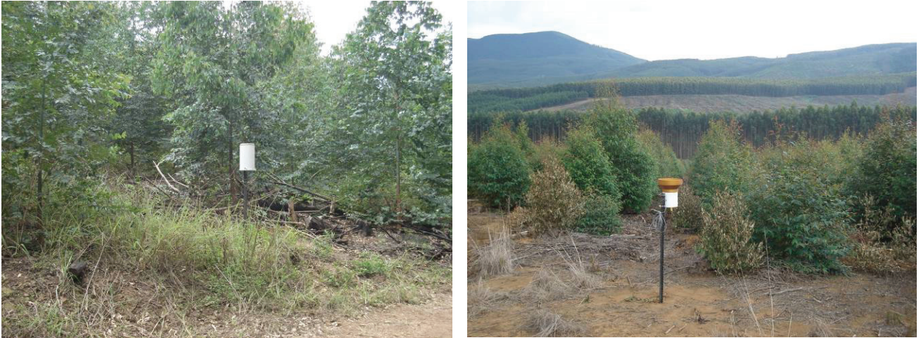
Figure 3.28. The upper and lower raingauges used to record the variability in rainfall within the catchment.
