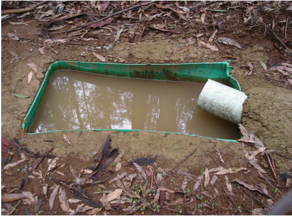
Figure 4.8. Blockage of the filter mesh by leaf litter at the inlet of the 110 mm pipe prevented the movement of water to the tipping bucket. This was solved for most plots by increasing the size of the mesh.
