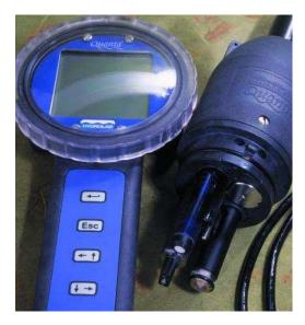
Figure 24. Hydrolab Quanta Probe (right) and hand-held control unit.
