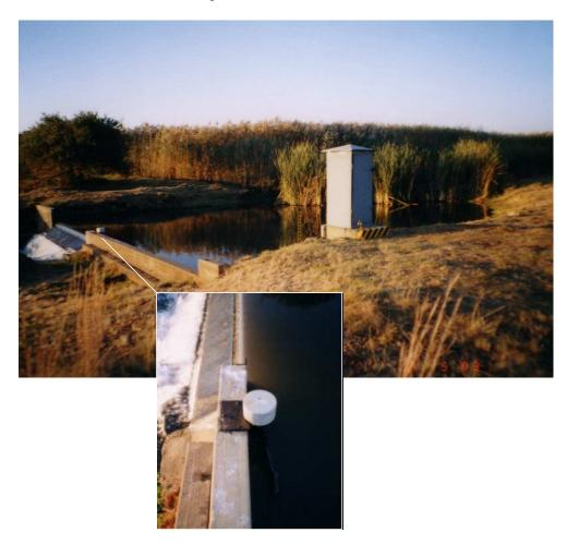
Figure 23. DWAF flow gauging station C2H069 at the Wonderfonteinspruit downstream of Welverdiend. Inset shows position of installed Hydrolab probe at the wall of the weir wired to a datalogger inside the gauging hut from where data were transferred to the Council for Geoscience via a cellular modem (Photos: Winde, 2003)
