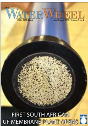
Cover: South Africa's first capillary ultrafiltration membrane production facility is now operational (See page 18).
