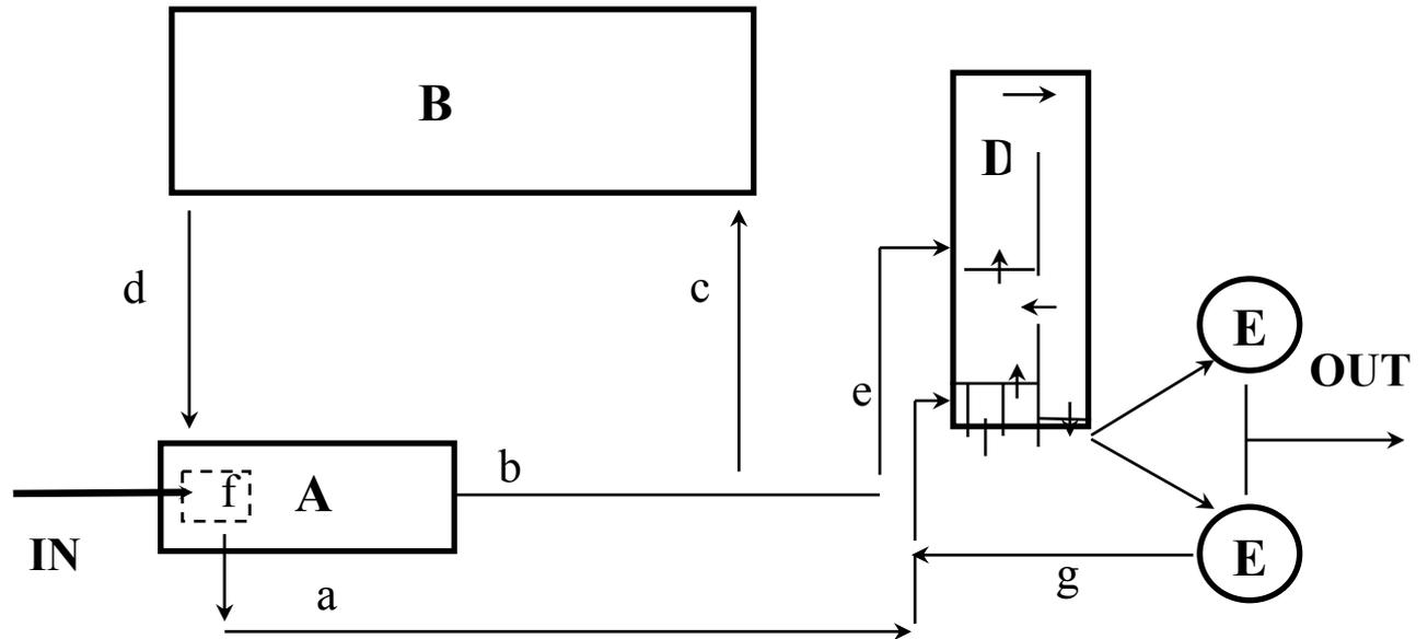
**Fig. 2. Basic PETRO BNR flow diagram. A. Primary pond; B. Secondary pond (s); D. PETRO BNR facility; E. Clarifiers; a. Extraction point for BNR anaerobic zone feed; b., e. Primary pond overflow (aerobic zone feed); c. Recycle to secondary pond(s); d. Algae-rich recycle (c : e+a, recycle ratio); f. The RBCOD Generating Pit; g. RAS.**
