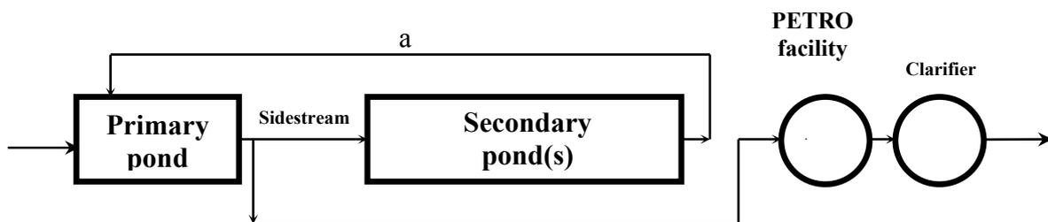
**Fig. 1. Basic flow diagram of the PETRO system. a: algae-rich recycle; PETRO facility is either an activated sludge reactor or trickling filter.**
