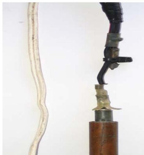
**Figure 10.2** Close-up of the probe at the end of the cable showing the upper bared end and the lower end soldered to the metal weight.
